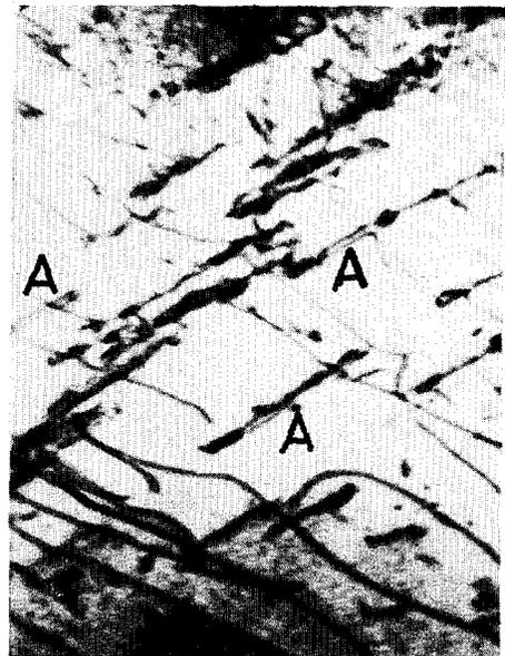
Fig. 9 Dipoles and elongated loop in 10% cold worked Zr
