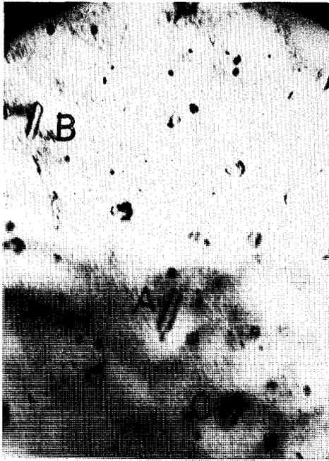
Fig. 18 Notice elongated loop contrast at A, B and C. (Irradiated Zr).
