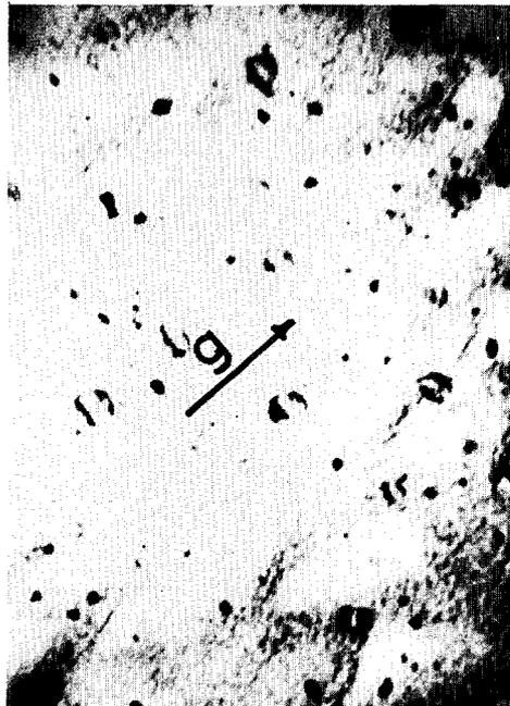
Fig. 20 General loop contrasts of defects in irradiated Zr
