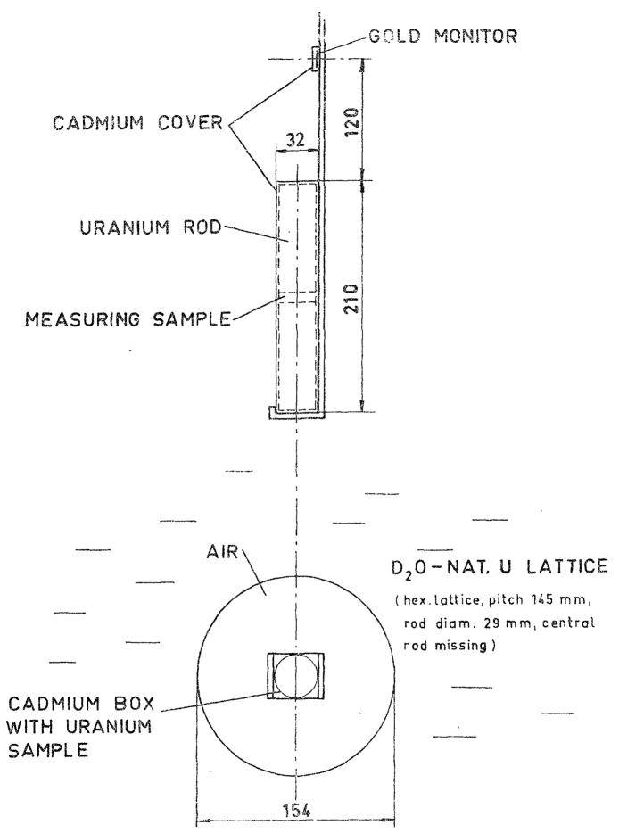
Fig. 1. Experimental arrangements
