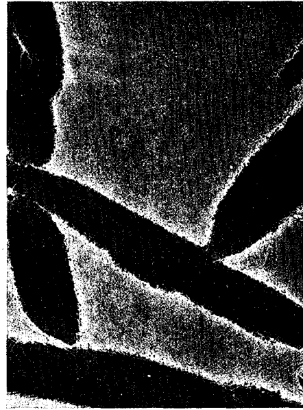
Fig. 19 b. 1050^{\circ} 12 min., 875^{\circ} 20 sec., w.q. electron microscope \times 2800 . Areas of beta at 875^{\circ} (light grey) between plates of alpha (dark grey).
