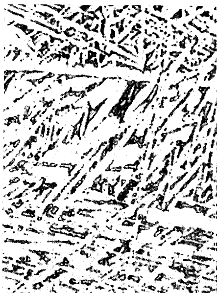
Fig. 17b. 1050^{\circ} 12 min., 700^{\circ} 2 sec., w.q. \times 2000 . Isothermally formed, fine alpha and beta (at 700^{\circ} ).
