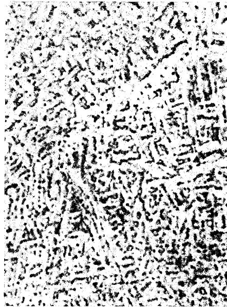
Fig. 26. 1050° 12 min., 500° 7 h 40 min., w.q. ×2000. X phase precipitated from supersaturated alpha.
