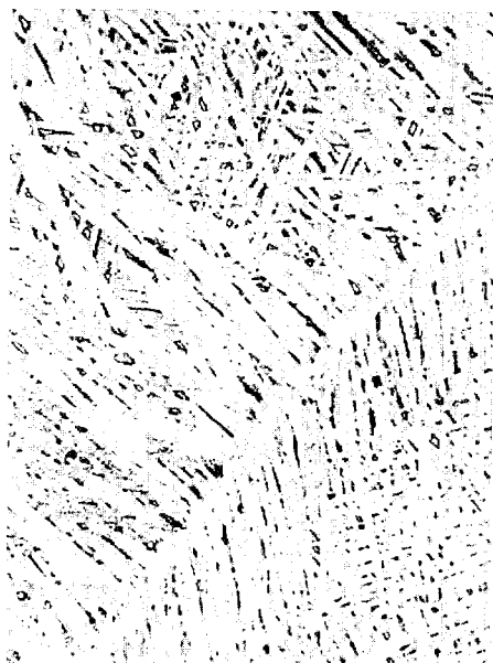
Fig. 16. 1050^{\circ} 12 min., 800^{\circ} 5 sec., w.q. \times 600 . Isothermally formed coarse alpha plates and fine plates formed during the quench. The small squares between alpha plates were beta at 800^{\circ} .
