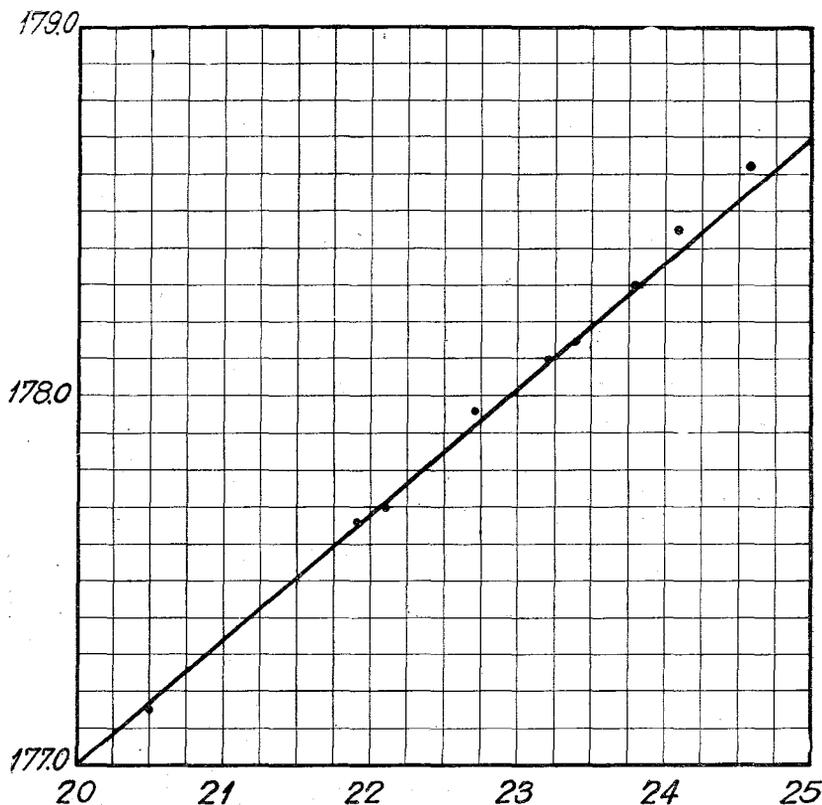
Diagr. 1. — The temperature dependence of the critical heavy water height.
