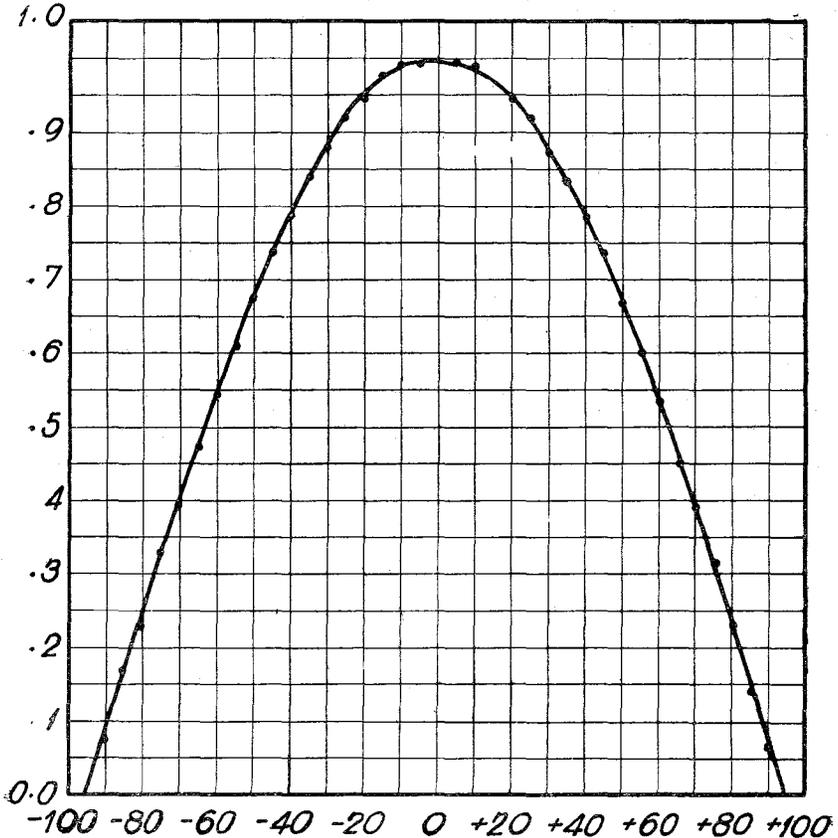
Diagr. 3. — The vertical thermal neutron flux distribution.
