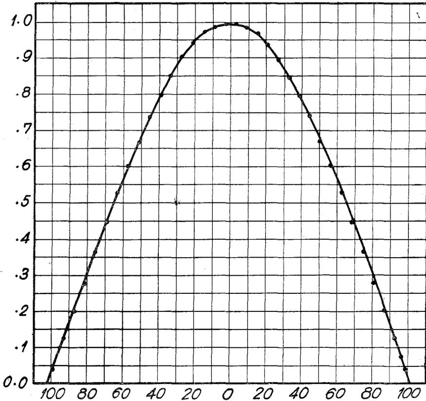
Diagr. 2. — The horizontal thermal neutron flux distribution.
