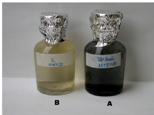
Figure 3: Growth of anaerobic consortium in medium containing 2,3,7,8 TCDD (A) and without microbes (B).
