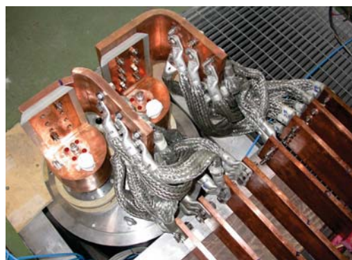
Fig. 4.7 - Connection between CERN 13-kA HTS leads and the bars of the ENEA power supply devoted to the test
