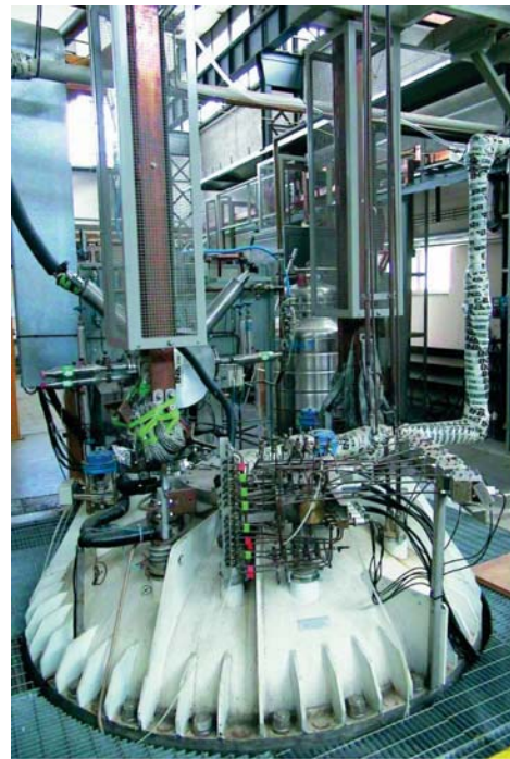
Fig. 4.6 - ENEA facility for testing superconducting solenoid magnets
