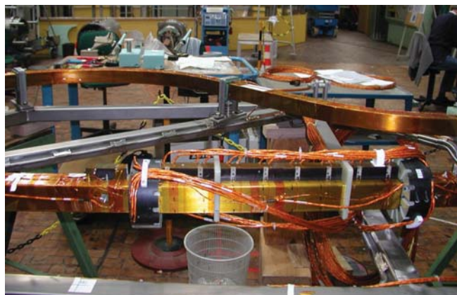
Fig. 4.4 - The BBIII full-size conductor with the Hall probe circular heads for current distribution measurements
