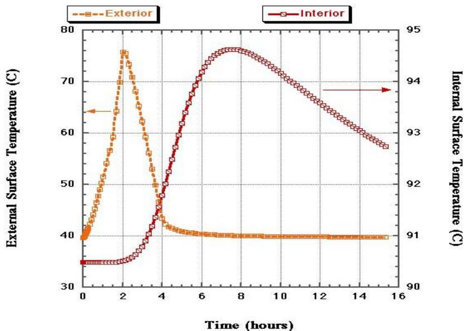
Figure 4. Plutonium package temperature response for a two-hour engine-room fire.
