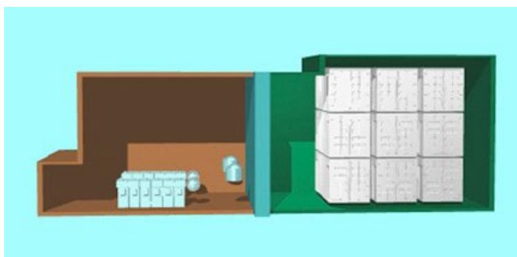
**Figure 3. Schematic drawing of the engine room and No. 5 Hold separated by a water-filled bulkhead.**
