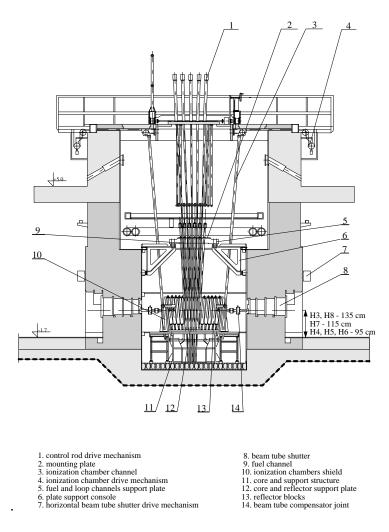
Fig. 1. Vertical section of MARIA reactor.
