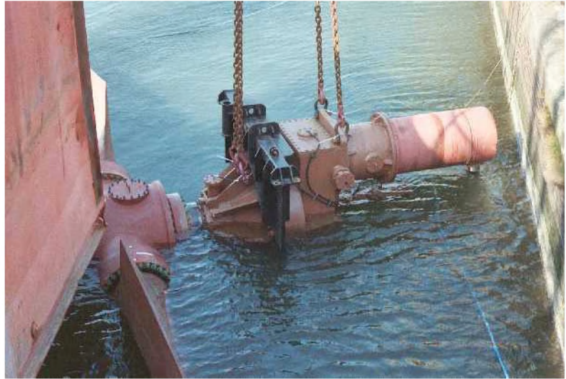
Figure 11: Submergence test for the powertrain on the quayside at Swansea.
