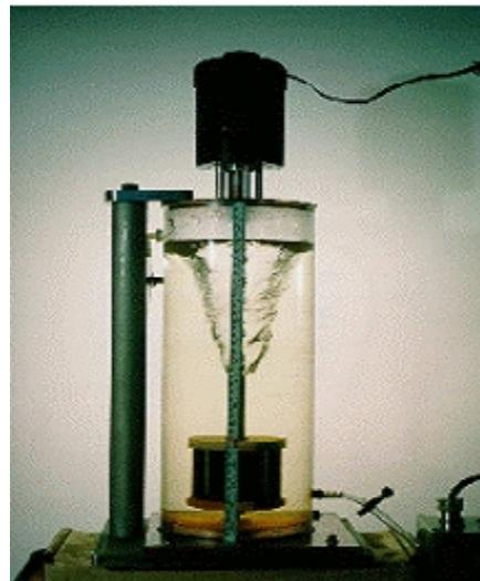
**Fig.1: Photograph of Rotating Cage**
