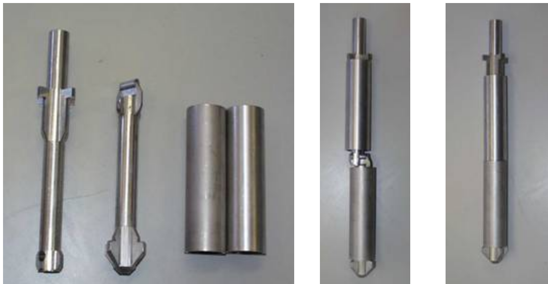
Figure 2: ANSTO prototype rig and annular targets for HIFAR
