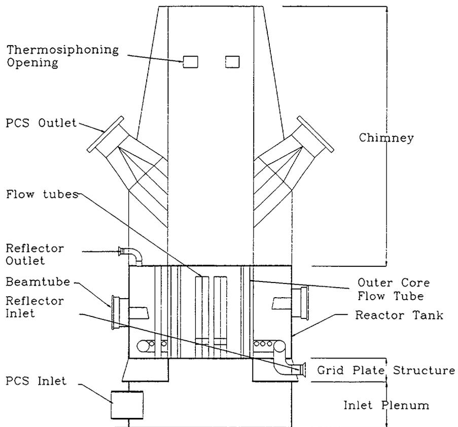
Fig. 1 Vertical View of the HANARO Reactor Assembly
