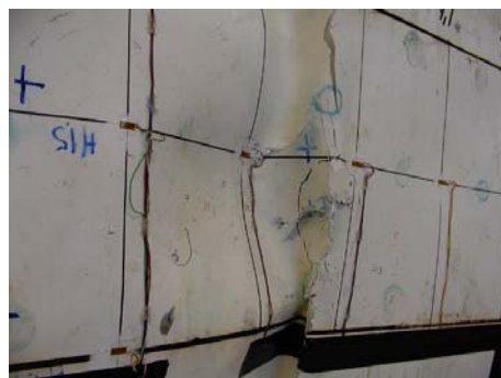
Figure 10 Test of section 3 with load introduction at 11.3m Figure 11 Failure 4.4m from the root.
