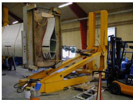
Figure 10 Test of section 3 with load introduction at 11.3m Figure 11 Failure 4.4m from the root.
