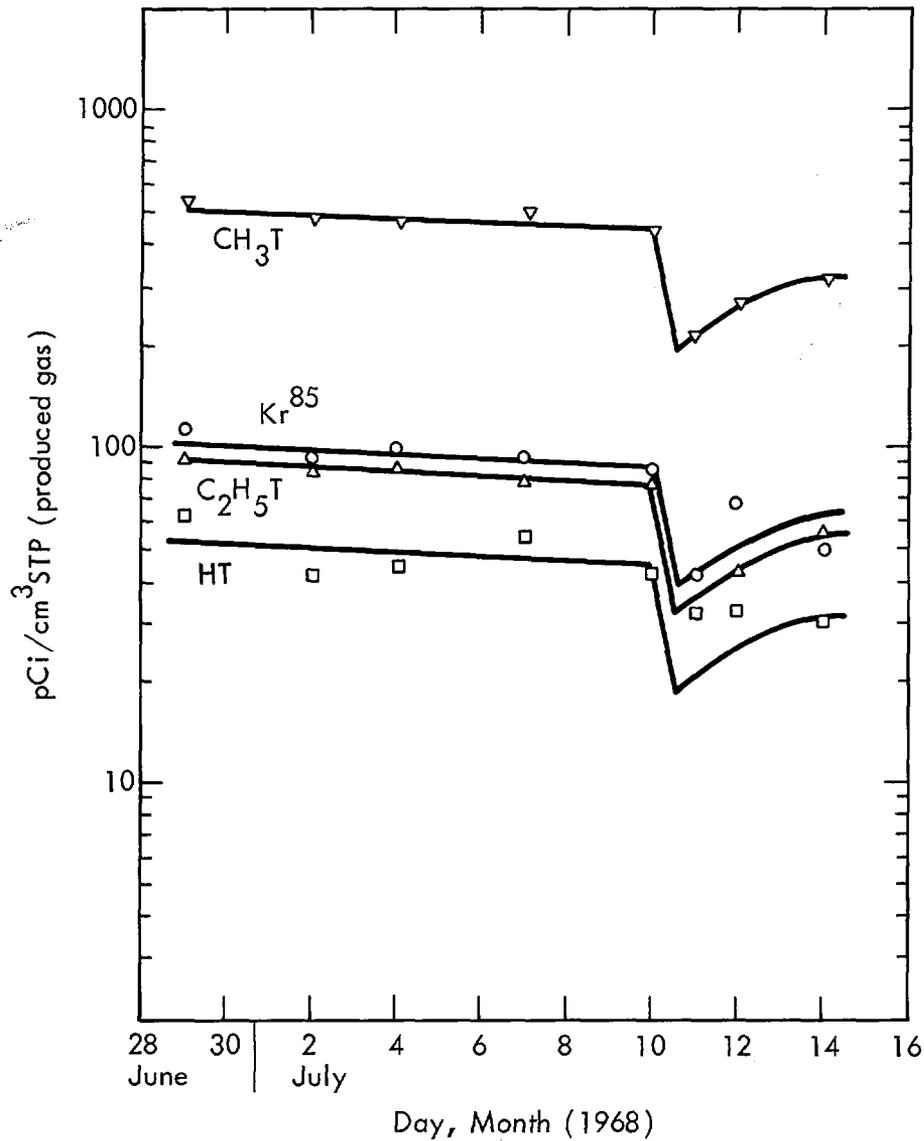
Fig. 6. High rate production test, radionuclide concentrations.
