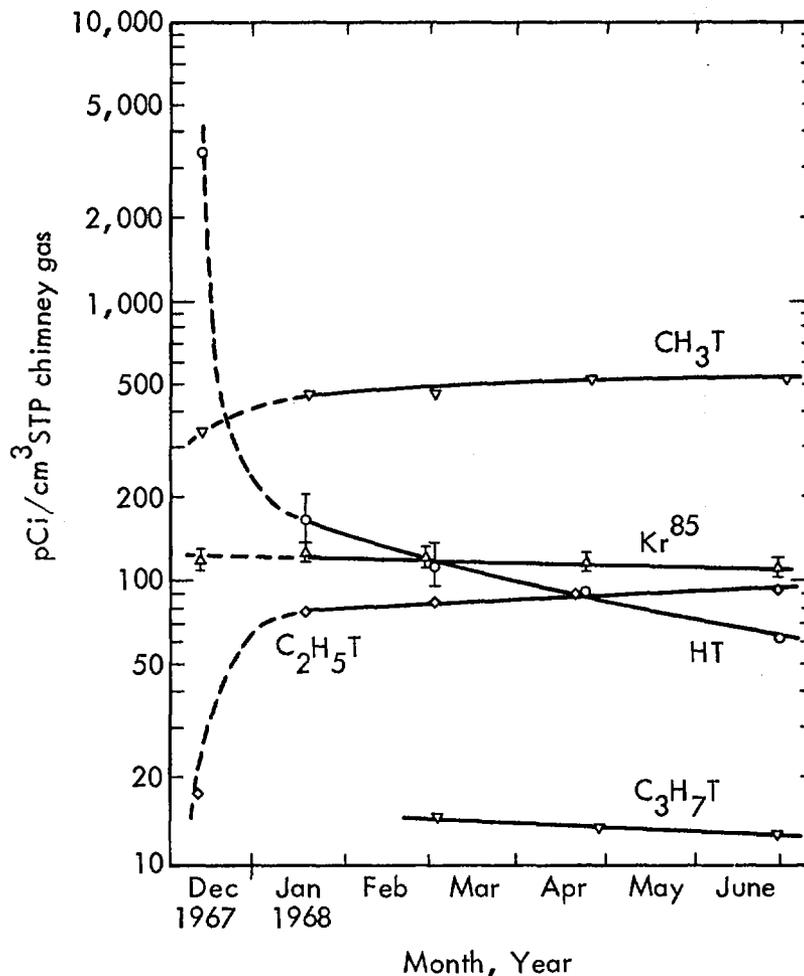
Fig. 3. Initial shut-in period, radionuclide concentrations.
