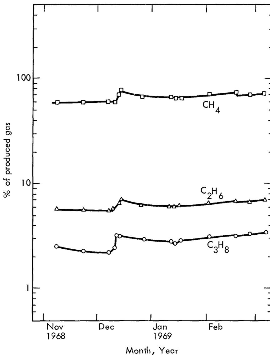
Fig. 7. Constant bottom hole pressure production tests, chemical composition.
