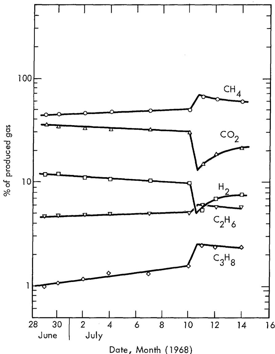
Fig. 5. High rate production test, chemical composition.
