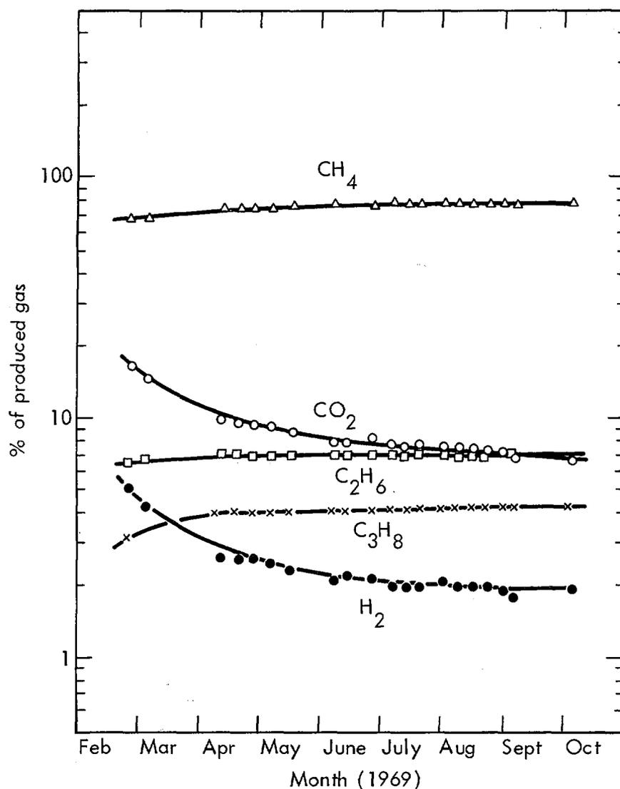
Fig. 10. Long-term production test, chemical composition.
