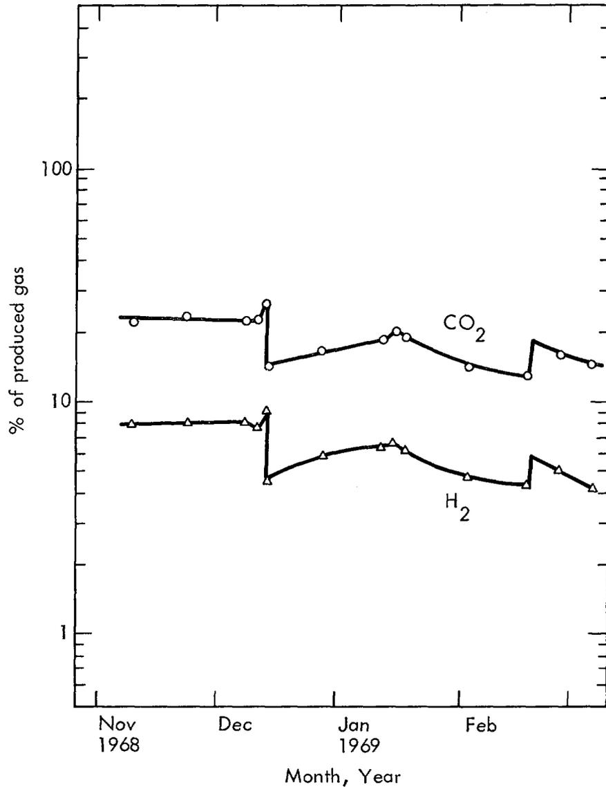
Fig. 8. Constant bottom hole pressure production tests, chemical composition.
