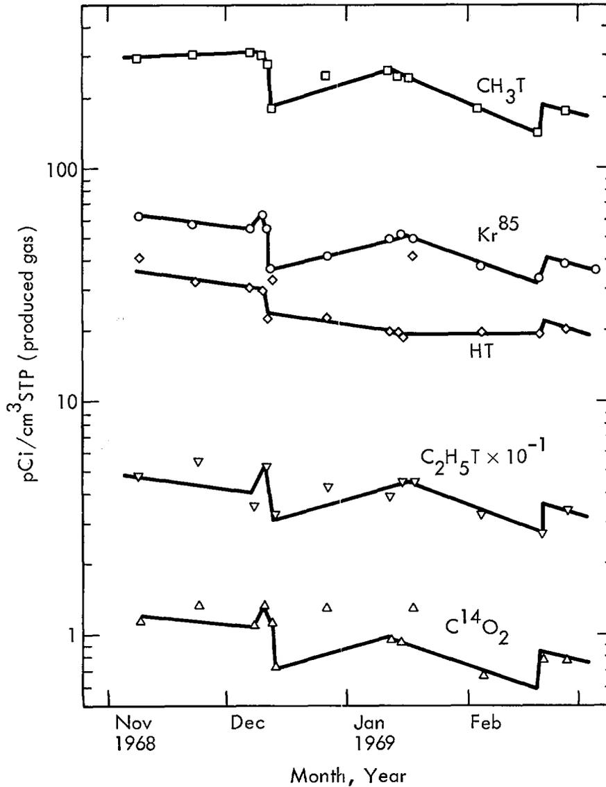
Fig. 9. Constant bottom hole pressure production tests, radionuclide concentrations.
