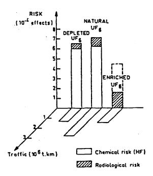
Fig. 2. Radiological and chemical accidental risk associated with the transport of  $UF_6$  in France in 1990.
