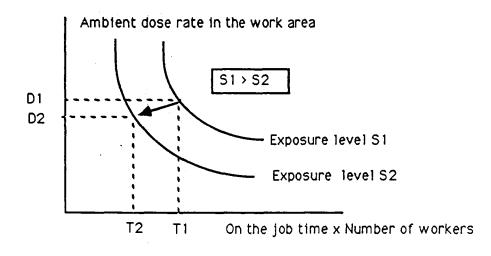
FIG.1. Impacts of robotics and remote tooling on basic parameters governing occupationnal exposures at nuclear facilities.
