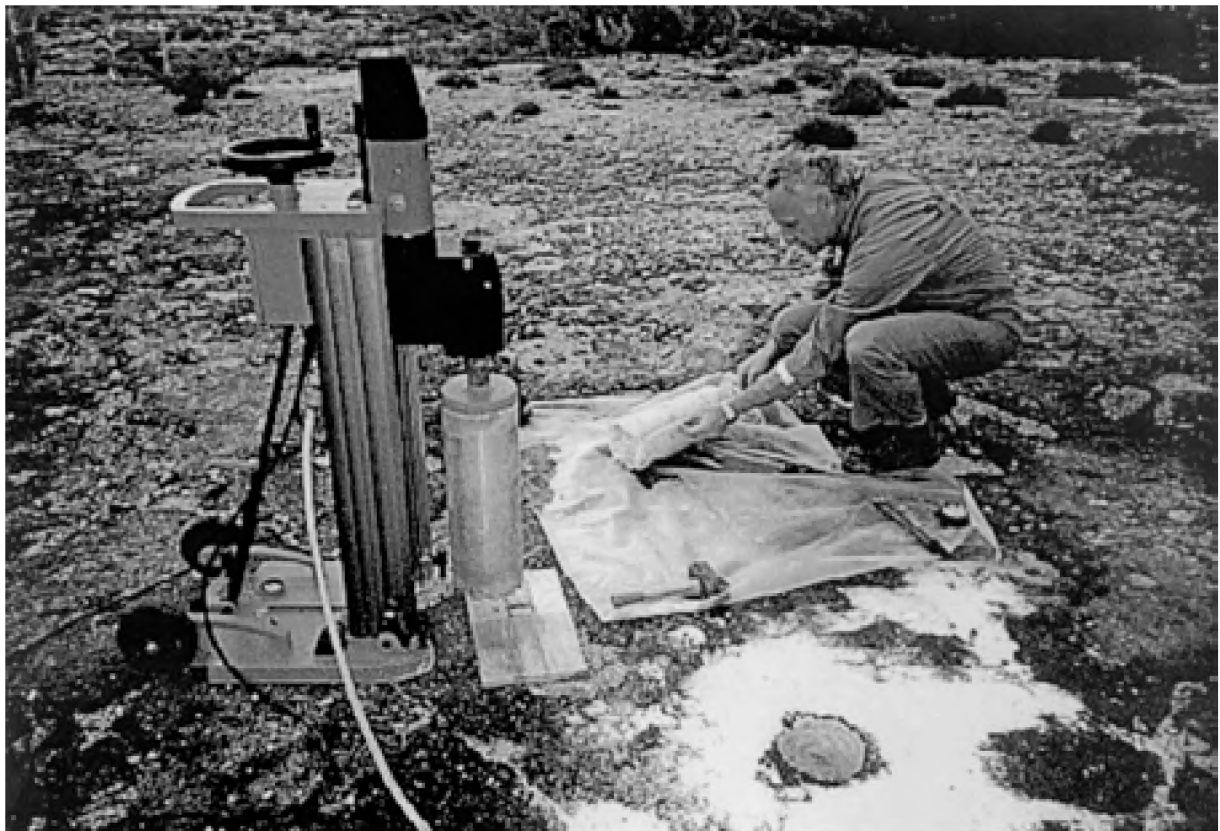
FIG 6: Bedrock sampling with core drilling equipment
