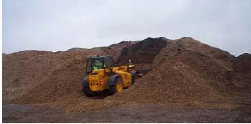
Plate 2. Interim sampling - using a teleporter to make a vertical face in the forestry residue pile
