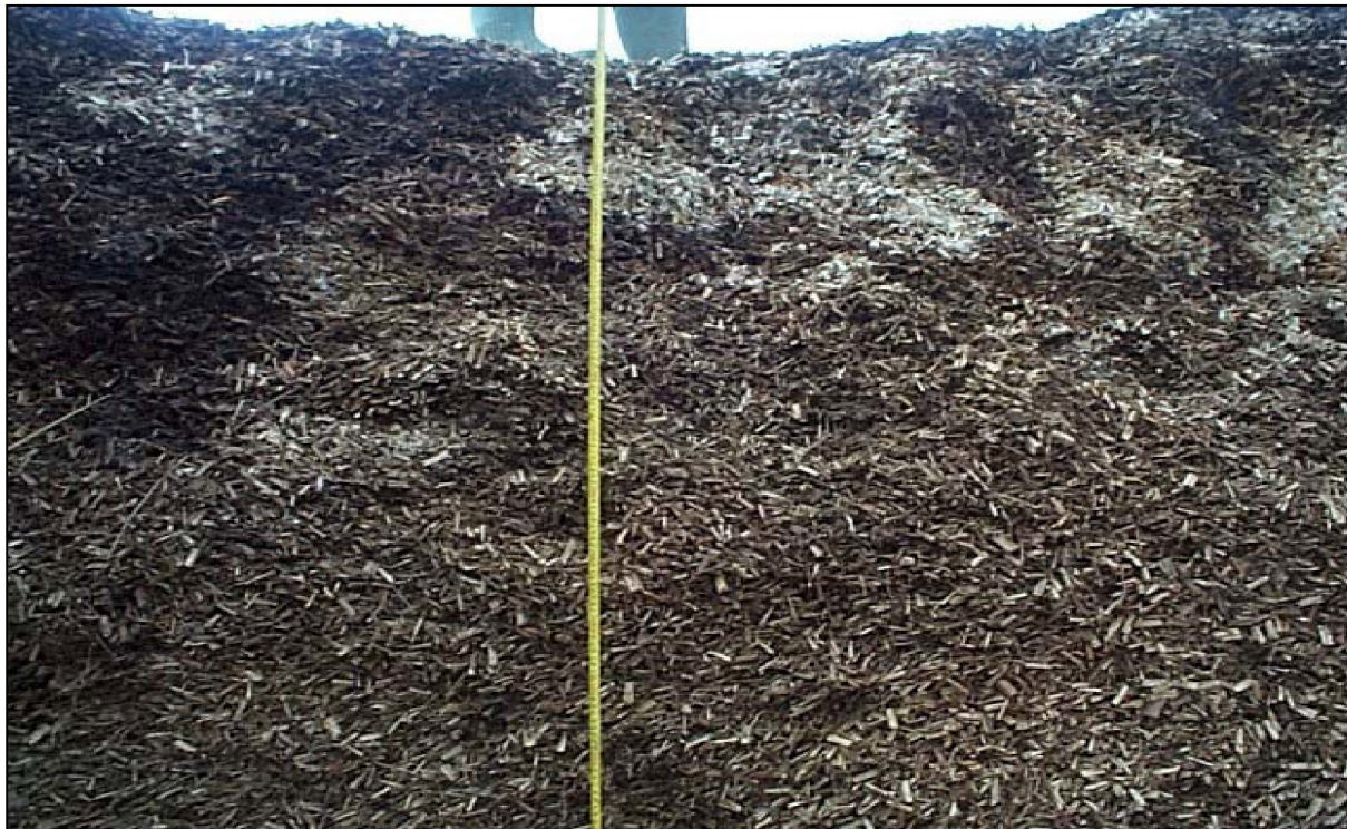
Plate 3. Fungal growth and subsequent chip degradation of SRC wood chip
