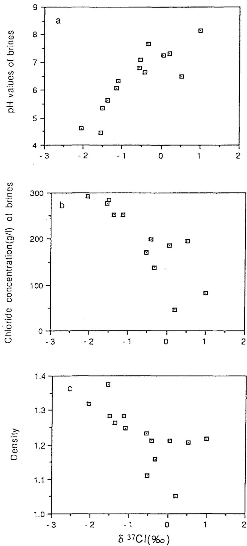
Fig. 4.7 Variation of  $\delta^{37}\text{Cl} (\text{\textperthousand})$  with: (a) pH; (b) chloride concentration; and (c) density of brines.<sup>61)</sup>
