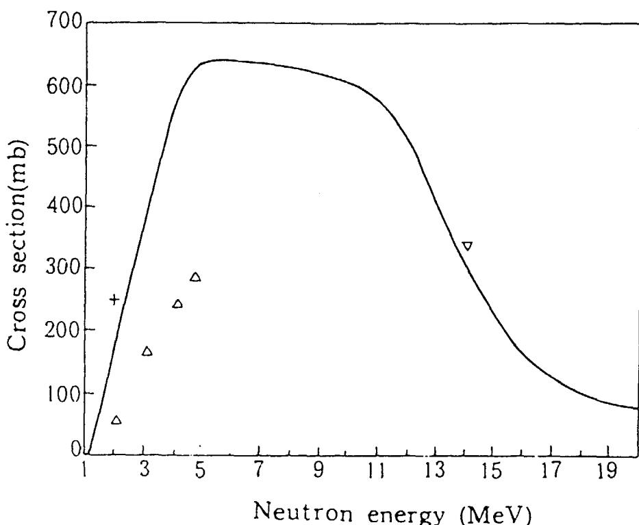
Fig. 5.9 The excitation curve of  $^{36}\text{Ar}(n,p)^{36}\text{Cl}$  reaction.<sup>104)</sup> △; Davis et al., +; Jiang et al., ; ▽; Levkovskii.
