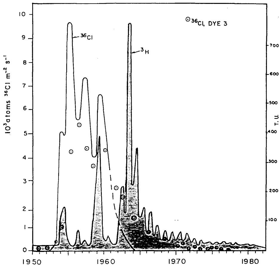
Fig. 5.3 A comparison of average northern hemisphere bomb  ${}^3\text{H}$  fallout, decay corrected to 1985, with calculated mean global bomb  ${}^{36}\text{Cl}$  fallout. The circles represent  ${}^{36}\text{Cl}$  fallout data from Dye 3 in Greenland. The measured  ${}^{36}\text{Cl}$  ( $\text{kg ice}^{-1}$ ) values were converted to  ${}^{36}\text{Cl}$   $\text{m}^{-2}$  assuming  $50 \text{ kg m}^{-2} \text{ y}^{-1}$  precipitation.<sup>93)</sup>
