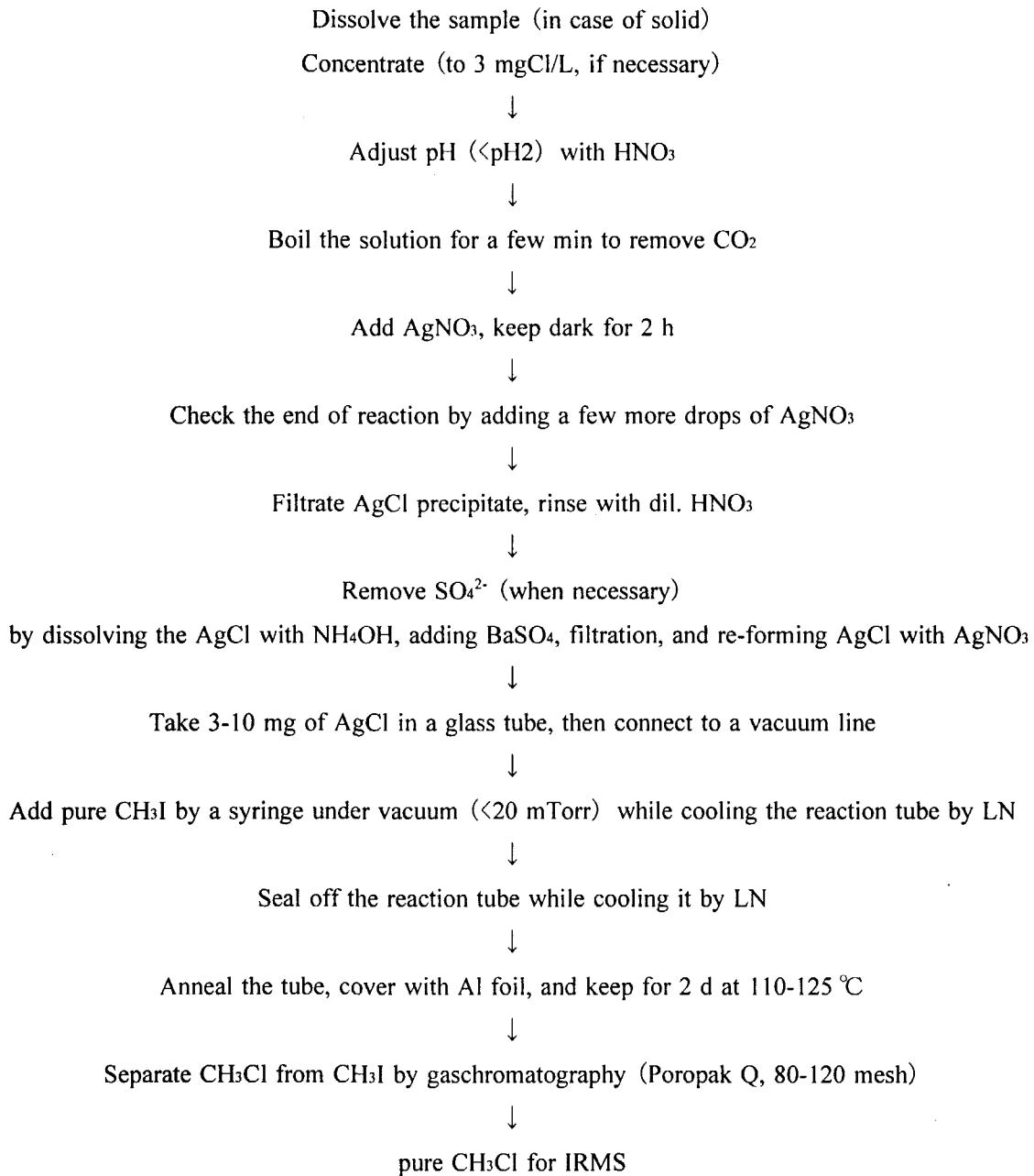
Fig. 6.3 Flow-sheet of chemical procedure for the synthesis of CH<sub>3</sub>Cl by Long et al.<sup>51)</sup>
