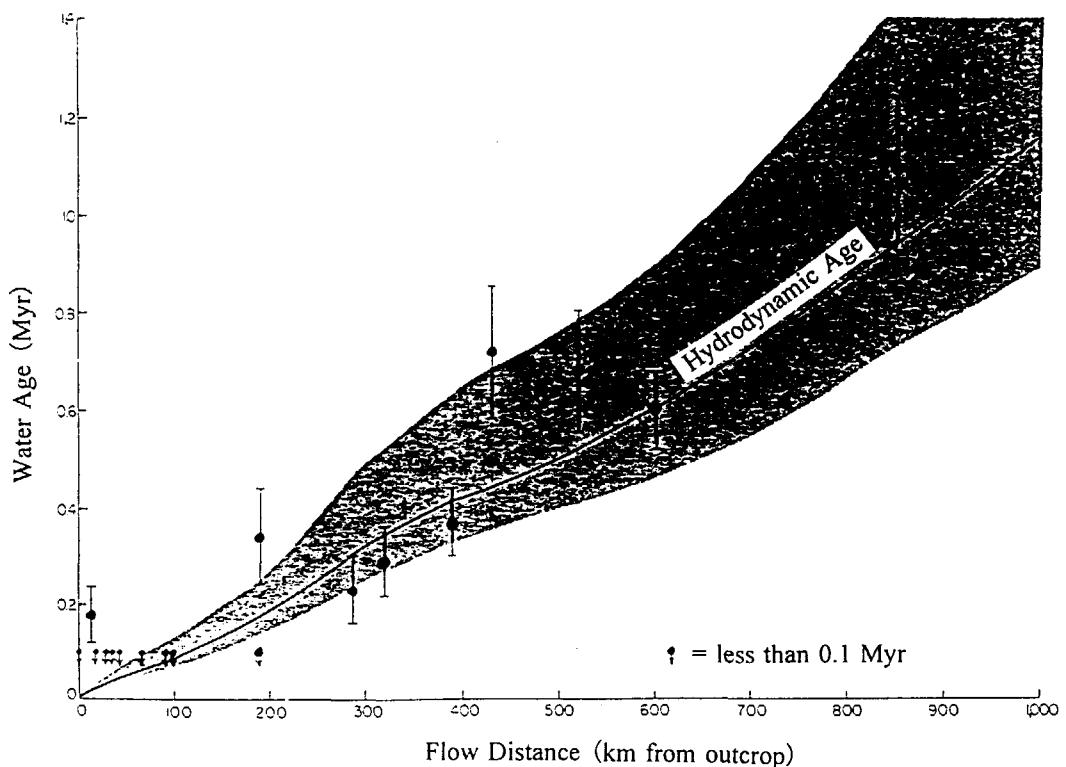
Fig. 5.14 Comparison of  $^{36}\text{Cl}$  and hydrodynamic groundwater ages along the southern flow line as a function of flow distance from the Hooray Sandstone outcrop.<sup>117)</sup> Shading around the hydrodynamic age line represents the age uncertainty resulting from an uncertainty of +50% and -25% in the ratio K/n.
