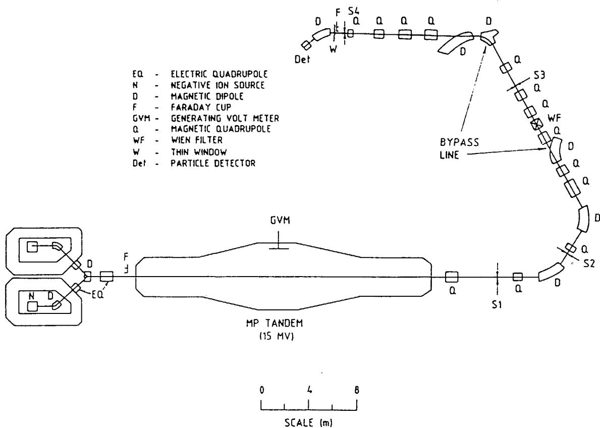
Fig. 5.1 Schematic diagram of the TASCC AMS facility.<sup>84)</sup>
