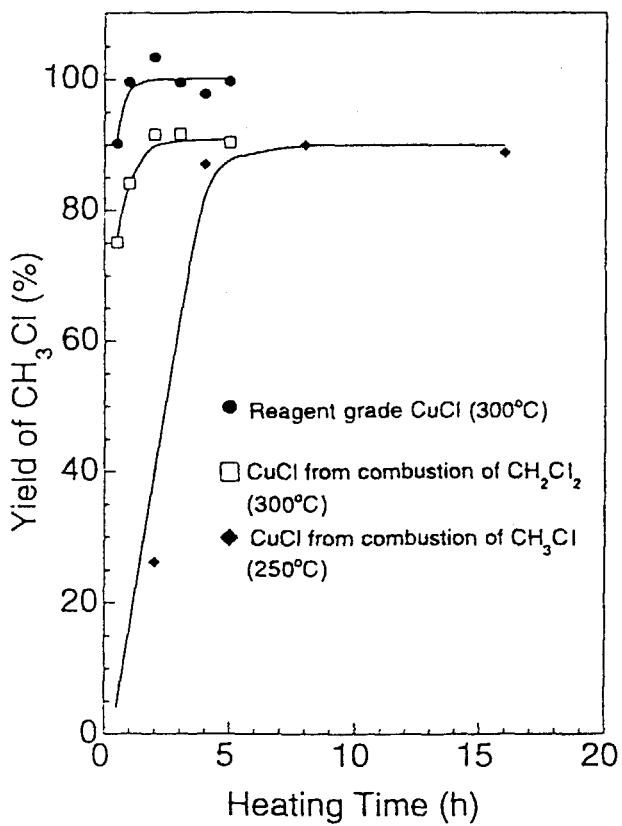
Fig. 4.5 Yield of  $\text{CH}_3\text{Cl}$  vs heating time for the reaction:  $\text{CuCl} + \text{CH}_3\text{I} \rightarrow \text{CuI} + \text{CH}_3\text{Cl}$ .<sup>54)</sup>
