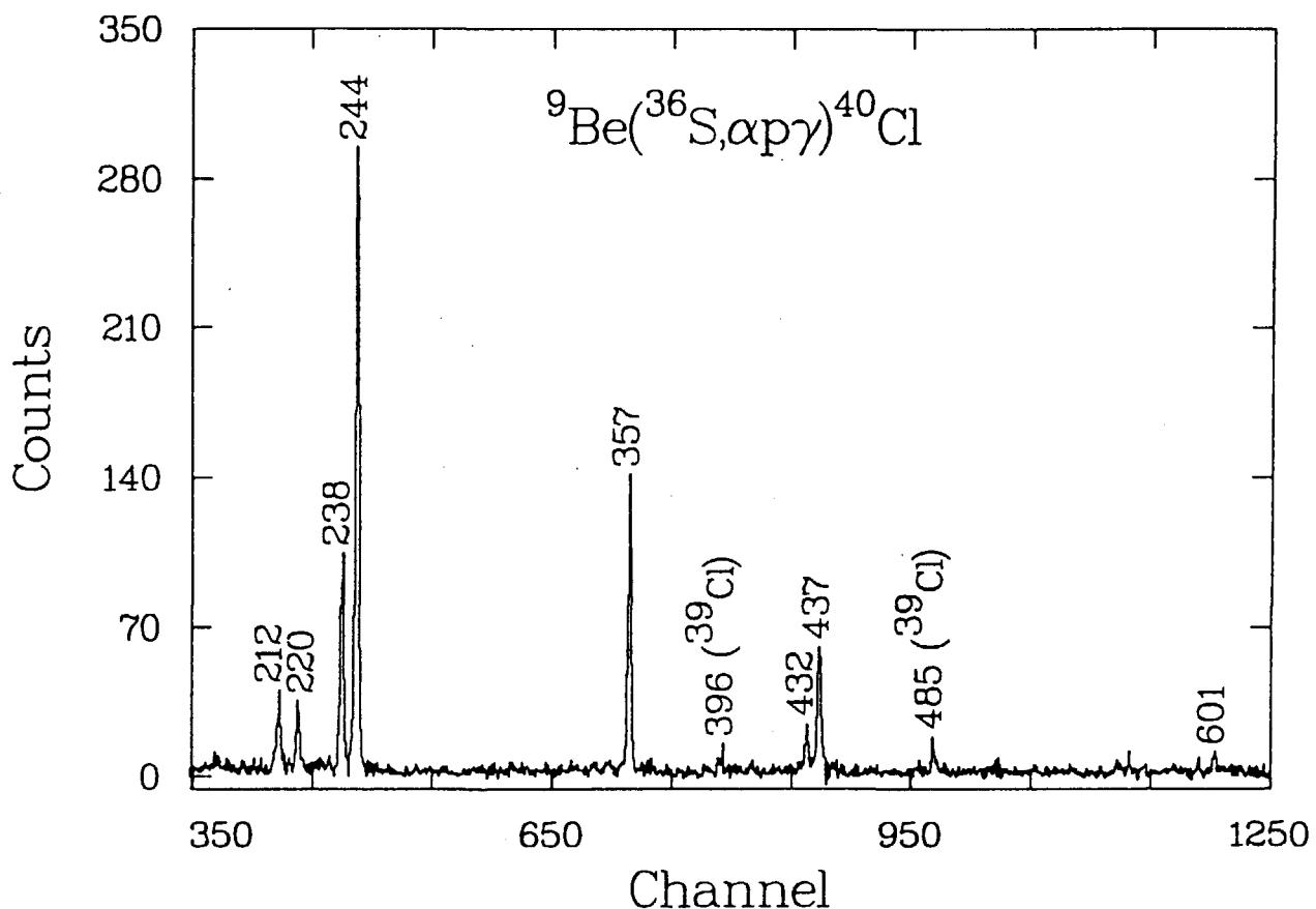
Fig. 5.18 Spectrum of  $\gamma$  rays in coincidence with an  $\alpha$  particle and a proton.<sup>133)</sup> All labeled lines are attributed to  $^{40}\text{Cl}$  unless otherwise noted. Energies are in keV. Random background from  $\alpha$  xn and pxn evaporation channels has been subtracted (note zero offsets).
