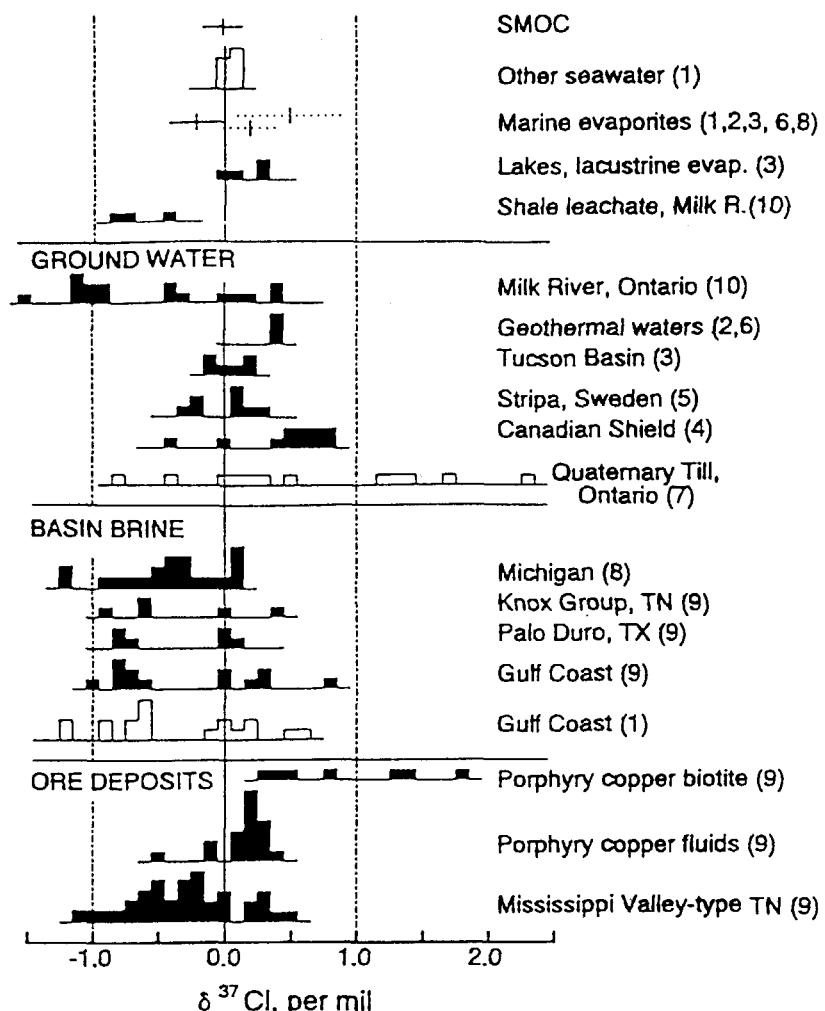
Fig. 4.4 Ranges of  $\delta^{37}\text{Cl}$  in natural samples studied.<sup>51)</sup> Data are presented as histograms or as mean  $\pm 2\sigma$ , where data are more numerous. For solid histograms and bars, precision =  $\pm 0.09\%$  ( $1\sigma$ ) or better. For others, precision =  $0.12\text{--}0.24\%$  ( $1\sigma$ ). Numbers in parentheses indicate references.
