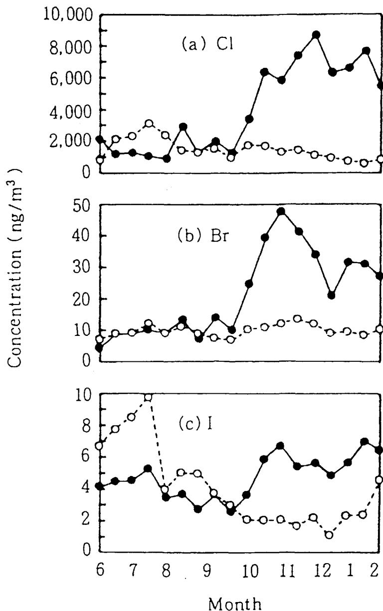
Fig. 2.1 Atmospheric particulate (●) and gaseous (○) Cl, Br and I concentrations from June 1991 to February 1992 in Chiba city, Japan.<sup>3)</sup>
