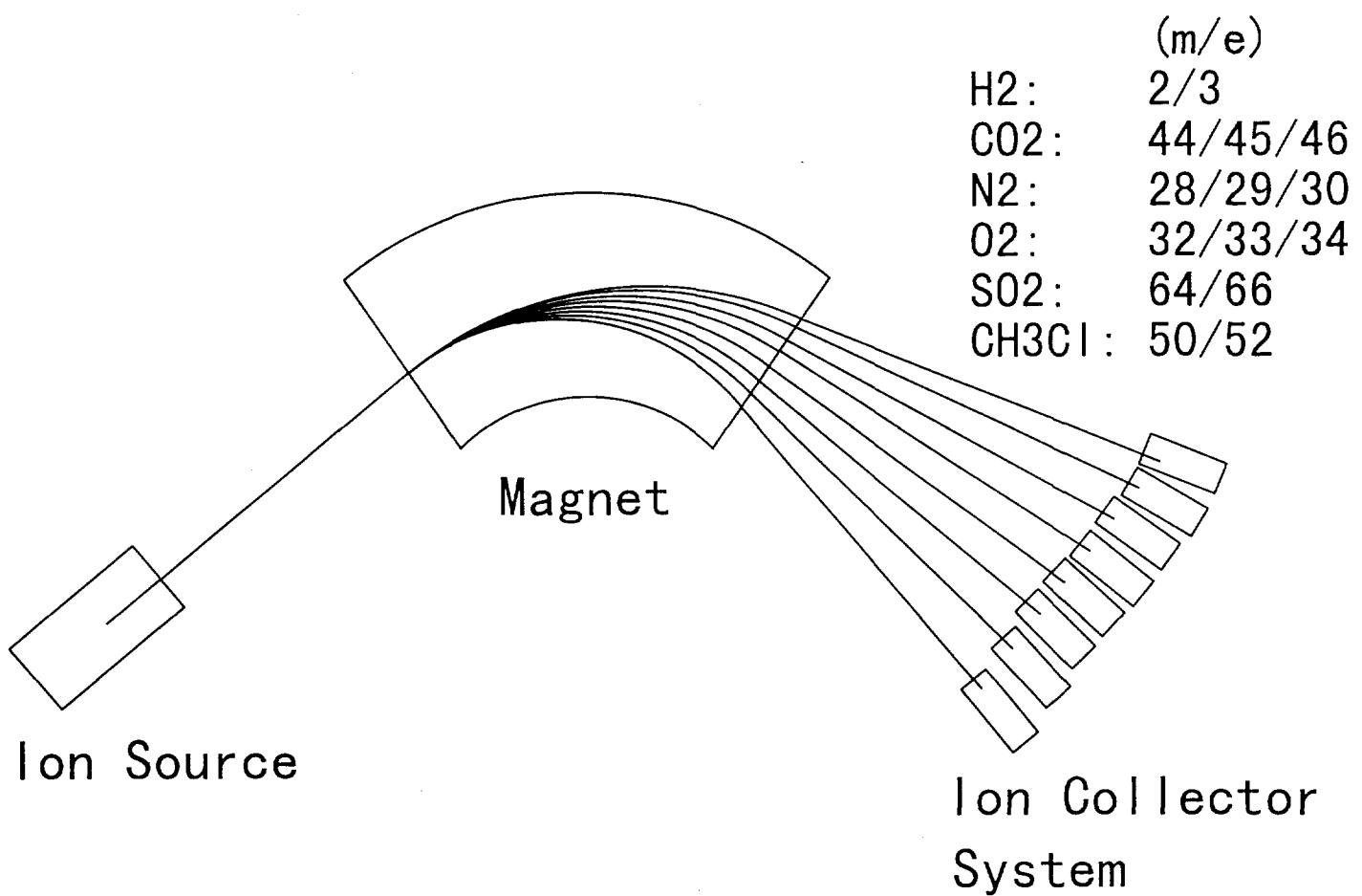
Fig. 6.1 Principle of isotope ratio mass spectrometry for the light elements.
