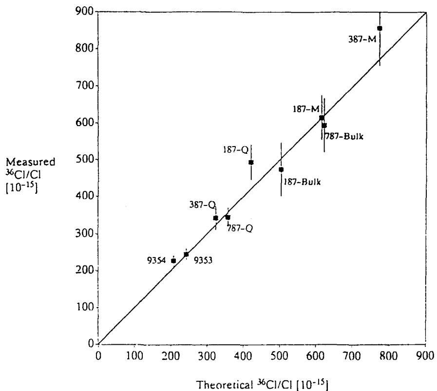
Fig. 5.12 Comparison of measured versus theoretically predicted  $^{36}\text{Cl}/\text{Cl}$  for the calibration samples.<sup>112)</sup>
