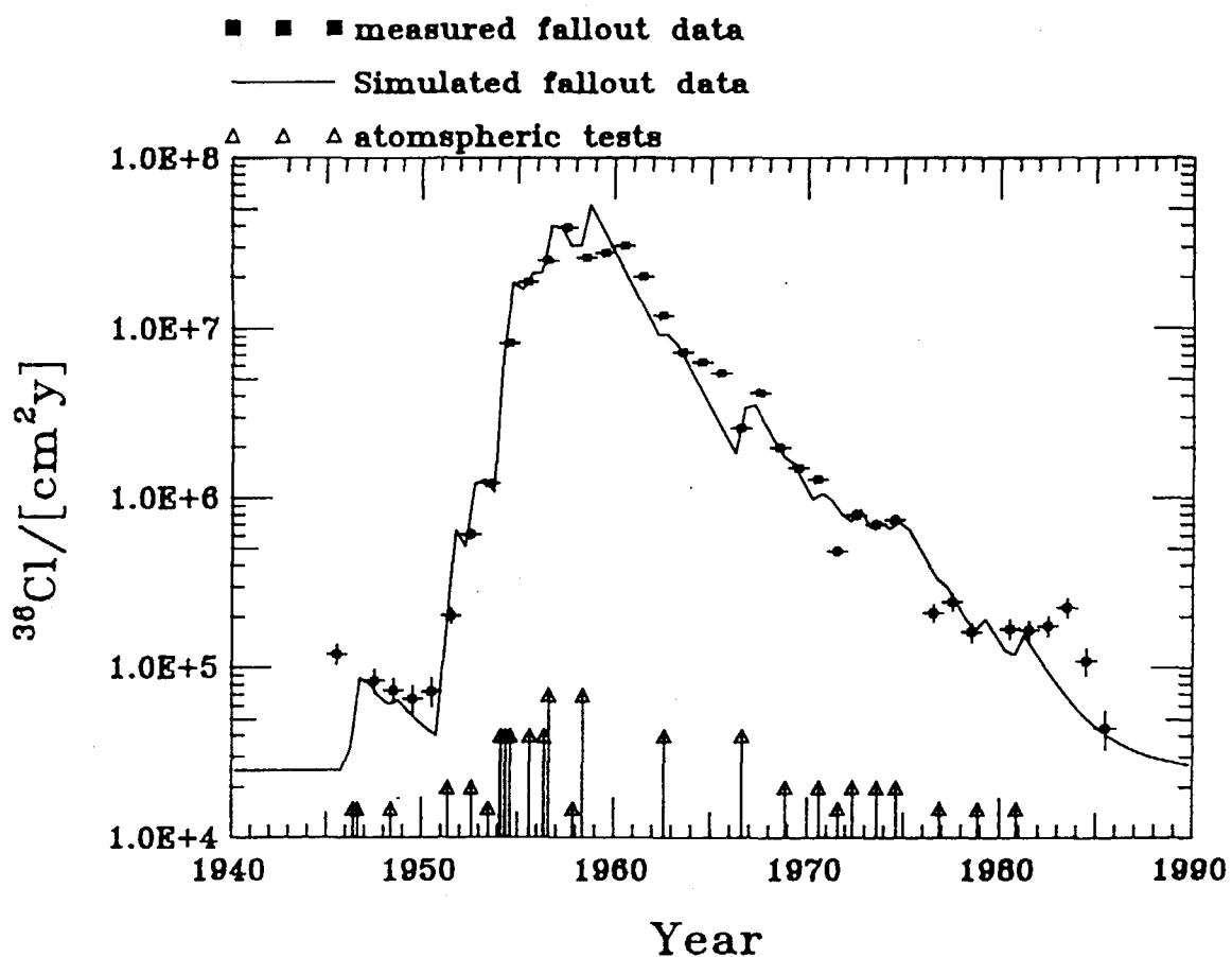
Fig. 5.4  $^{36}\text{Cl}$  fallout rates are compared with the results from model calculations.<sup>94)</sup> For the calculations a  $^{36}\text{Cl}$  stratospheric residence time of 2 years has been used. The arrows indicate the dates when  $^{36}\text{Cl}$  release to the atmosphere has been considered.
