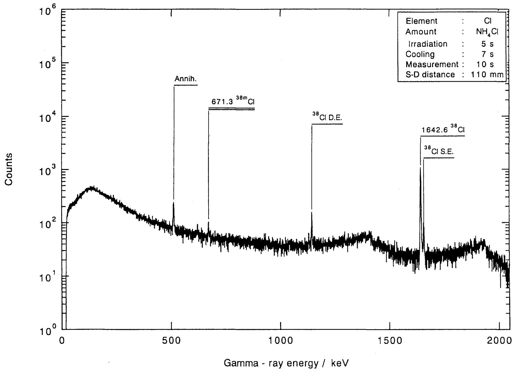
Fig. 5.17 Gamma-ray spectrum of irradiated  $\text{Cl}^{129}$ )
