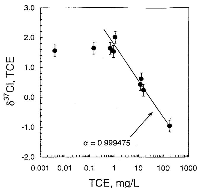
Fig. 4.11 Diagram showing  $\delta^{37}\text{Cl}$  value of TCE (‰) vs TCE concentration (mg/L) in water samples.<sup>80)</sup> Solid line is exponential best-fit yielding  $\alpha = 0.999475$ .
