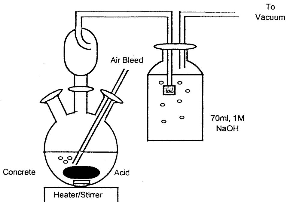
Fig. 5.8 Apparatus used for the digestion and separation of chlorine and iodine from concrete.<sup>101)</sup> In the extraction flask, NaCl and NaI carrier are added to 3 M nitric acid at 70 °C to extract iodine. After 3 h, potassium permanganate solution is added to the flask at 70 °C to extract chlorine. To the sodium hydroxide solution containing chlorine, sodium nitrite solution is added to reduce chlorate to chloride, then silver nitrate solution is added to precipitate silver chloride.
