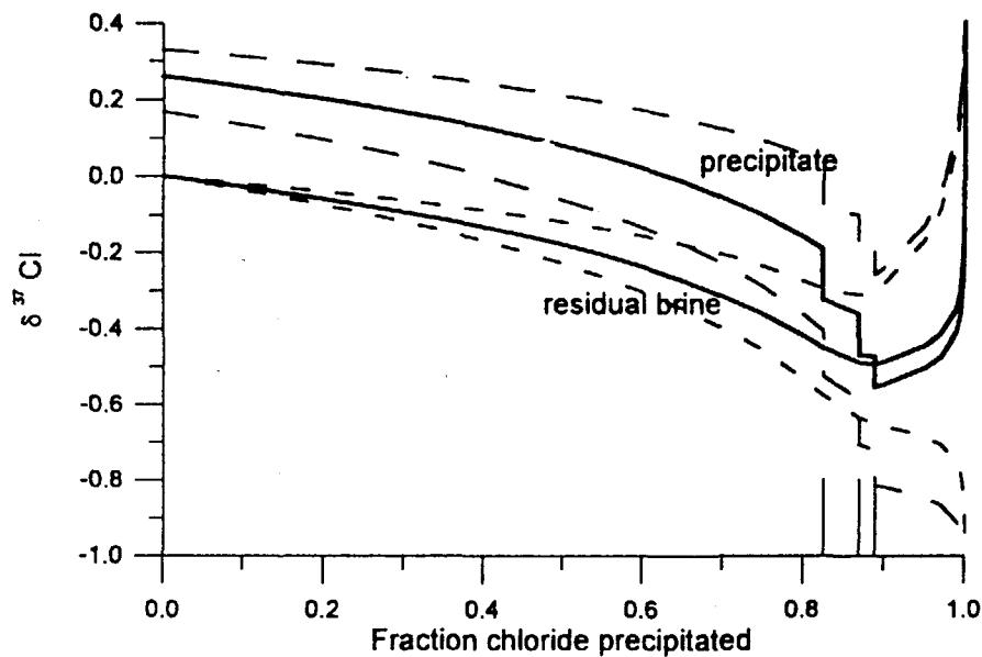
Fig. 4.8 Calculated  $\delta^{37}\text{Cl}$  values of the precipitate and the remaining brine.<sup>66)</sup> The bold lines indicate the average values. The area between the short-dashed lines indicates the error for the residual brines and the area between the long-dashed lines indicates the error for the precipitates. Note the discontinuities in the curves for the precipitates.
