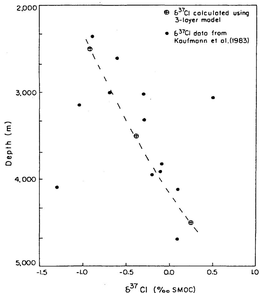
Fig. 4.10 A comparison of calculated  $\delta^{37}\text{Cl}$  as a function of depth<sup>77)</sup> with data obtained by Kaufmann et al.<sup>37)</sup>
