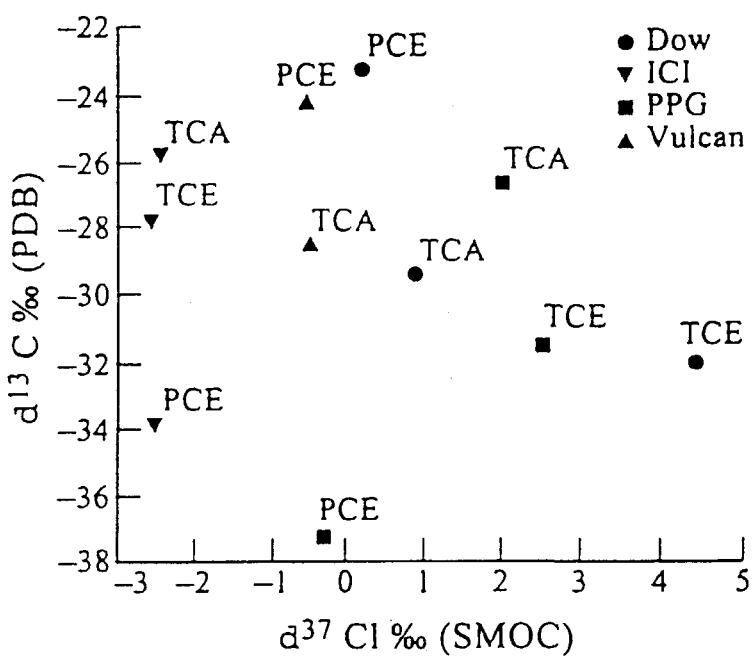
Fig. 4.12  $\delta^{37}\text{Cl}$  vs  $\delta^{13}\text{C}$  of PCE, TCE and TCA from 4 different manufacturers.<sup>83)</sup> The solvent type is noted beside the isotopic field: Dow; Dow Chemical Company, ICI; ICI Chemicals and Polymers Group, PPG; PPG Industries, Vulcan; Vulcan Chemicals.
