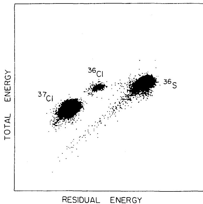
Fig. 5.2 Two-dimensional plot of total energy versus residual energy measured by the detector, showing the separation of  $^{36}\text{Cl}$  from  $^{36}\text{S}$  and  $^{37}\text{Cl}$  ions.<sup>84)</sup>
