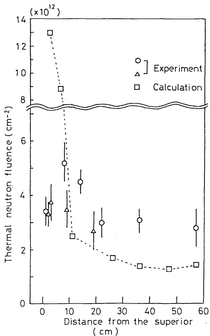
Fig. 5.6 Thermal neutron fluence in the upper part of the tombstone.<sup>97)</sup> The ordinate indicates the thermal neutron fluences derived from the  $^{36}\text{Cl}/\text{Cl}$  ratios on the assumption that  $^{36}\text{Cl}$  were produced only by thermal neutrons. The squares show results obtained from a preliminary Monte Carlo calculation for Pace's neutron fluence, where the energy output of the A-bomb assumed to be 15 kilotonnes.)
