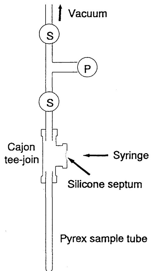
Fig. 4.2 Vacuum line for the preparation of  $\text{CH}_3\text{Cl}$ .<sup>51)</sup> S = stopcock, P = pressure gauge.
