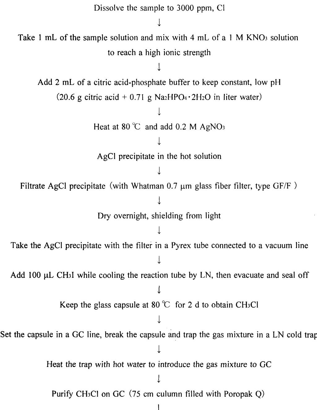
Fig. 6.4 Flow-sheet of chemical procedure for the synthesis of  $\text{CH}_3\text{Cl}$  by Eggenkamp et al.<sup>53, 66)</sup>
