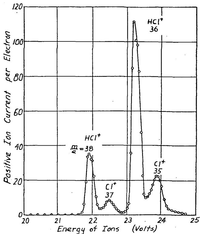
Fig. 4.1 Typical mass spectrum found in the region of  $HCl^+$ . Accelerating voltage applied to electrons was 100 V, and magnetic field was 1175 gaus.<sup>43)</sup>
