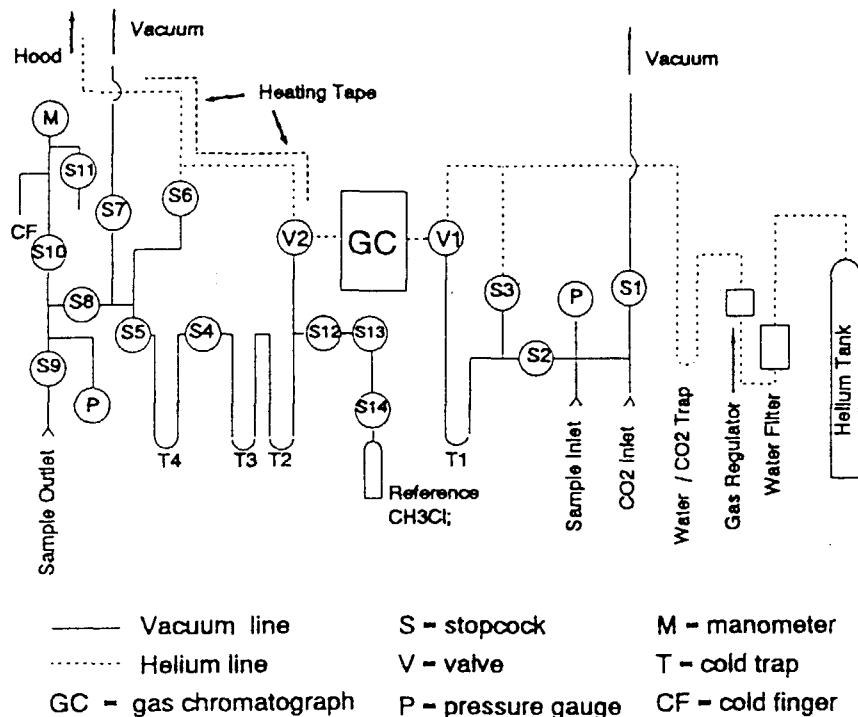
Fig. 4.3 Vacuum line for the purification of  $\text{CH}_3\text{Cl}$ .<sup>51)</sup>
