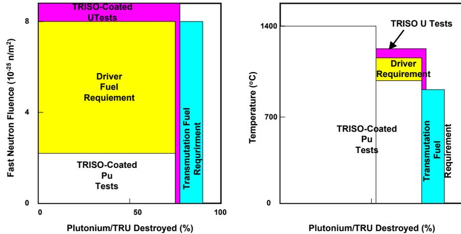
Figure 6. Comparison of DF and TF Requirements with the Irradiation Database
