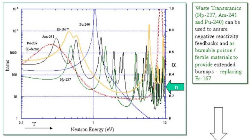
Figure 3: Capture cross-sections of selected minor actinides
