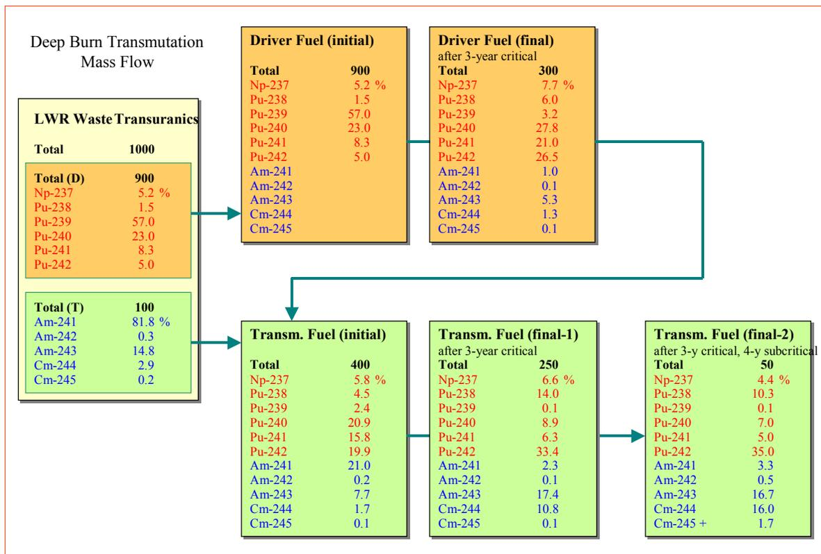
Figure 4 From LWR Waste to Final Waste after Deep Burn Transmutation: mass flow results from the Deep Burn Transmuter studies. The mass flow of the wastetransuranics is followed through the Driver and Transmutation Fuel stages, the critical (MHR&T) and subcritical (MHA&T) irradiation periods.
