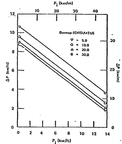
Figure 2. Predicted Change-In-Power ( $\Delta P$ ) Failure Boundaries as a Function of Irradiation Power ( $P_1$ )
