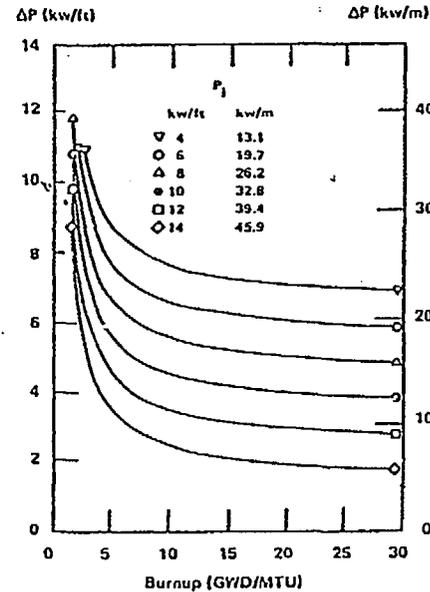
Figure 1. Predicted Change-In-Power ( $\Delta P$ ) Failure Boundaries as a Function of Burnup
