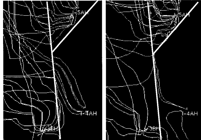
Figure 4. Effect on streamline patterns by closing the north-south fault and opening the east-west fault. Left: original model. Right: model modified by fault transmissibility multipliers.
