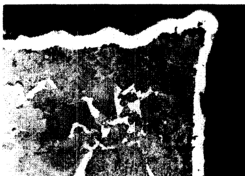
Fig. 8. Sectional view of an edge with vanadium carbide coating
