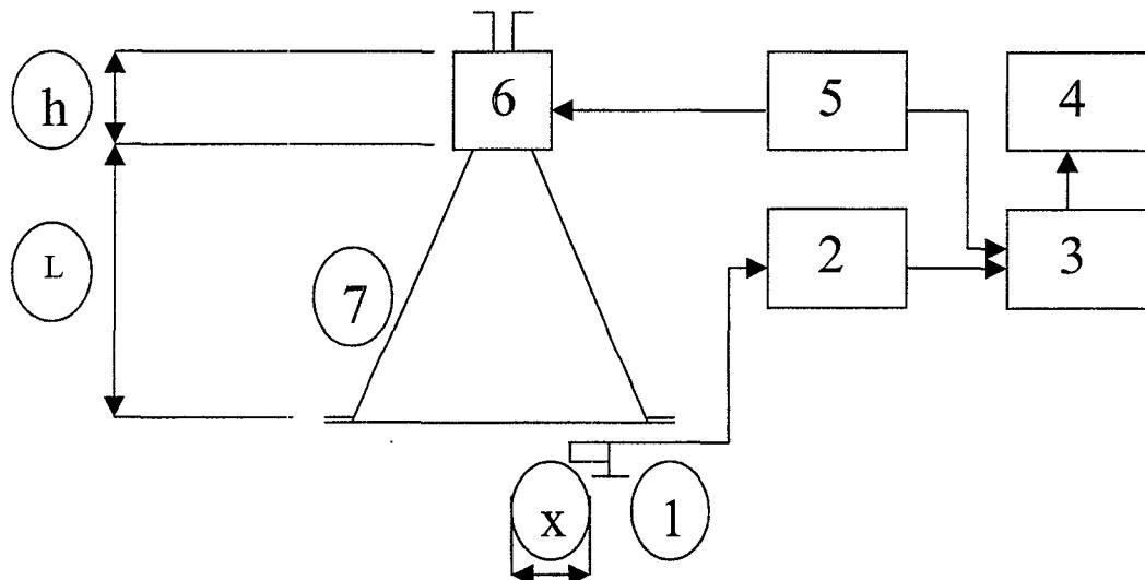
A secondary electrons monitor for continuous electron energy measurements described in this paper is based on application of scanned electron beam which is typically used in industrial facilities devoted to radiation sterilization process. The principal idea of the measurements is
