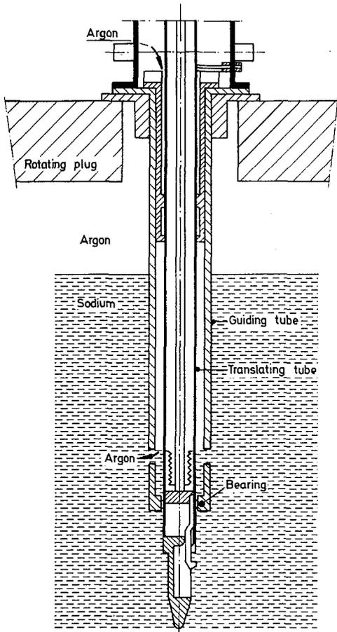
PHENIX - CONTROL ROD MECHANISM
