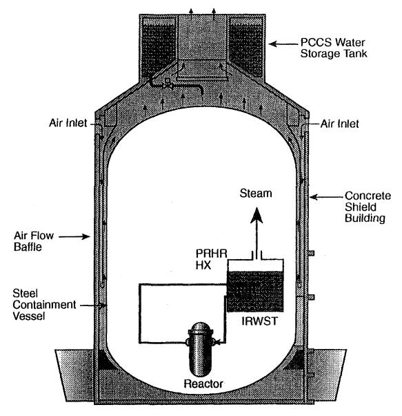
FIG. 2. AP600 Plant Heat Sink
