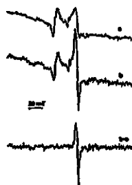
Figure 3. EPR spectra of \text{TiO}_2 , P25 powder: a) non-irradiated b) irradiated 1 minute b-a) numerical subtraction of the spectrum a from spectrum b
