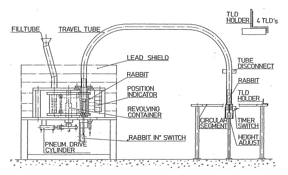
Fig. 12: Schematic View of Circular Exposure System
