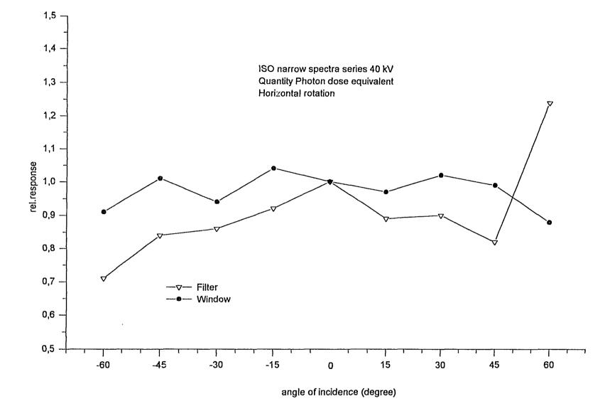
Fig. 11: Directional Response at 33 keV - Horizontal Rotation
