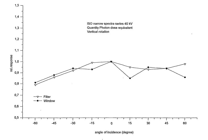
Fig. 10: Directional Response at 33 keV - Vertical Rotation
