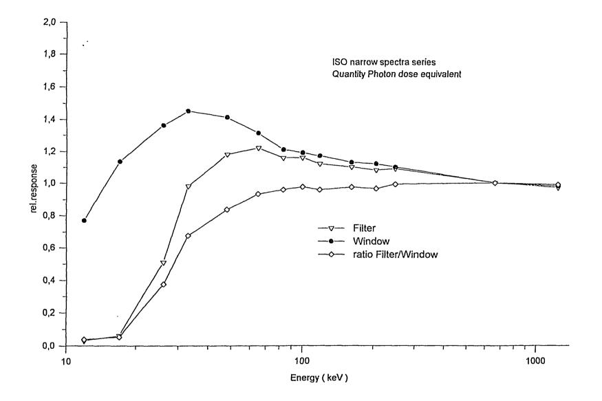
Fig.8: Energy Response of filtered and unfiltered TL element and ratio
