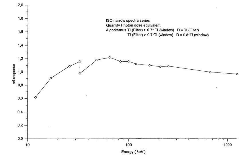
Fig. 9: Energy Response of dosimeter with readout algorithm applied
