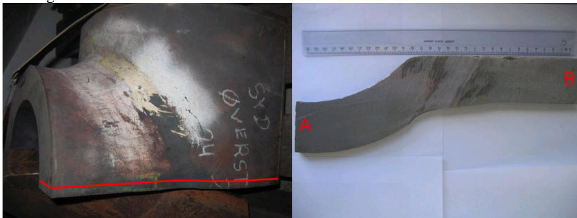
Sectioning of branch joint and position of material used for LOM and TEM
