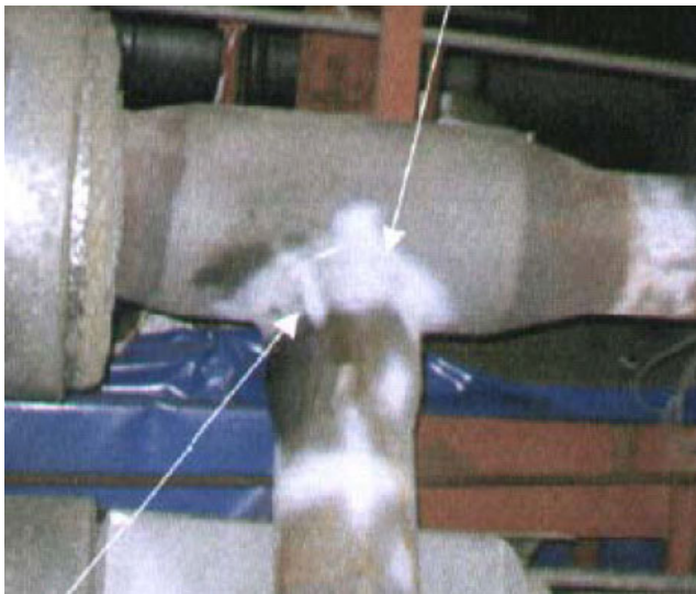
Branch connection RA11. Arrows at standard replica position and ground indication.
