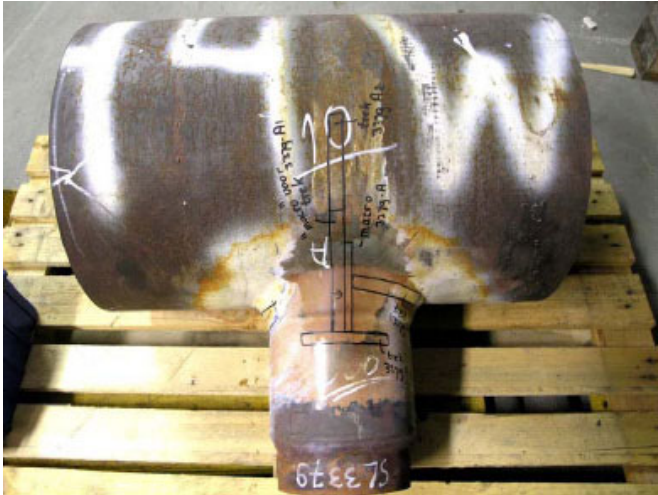
GLD13 Header 600, Nozzle 10, side A. Location of samples for testing
