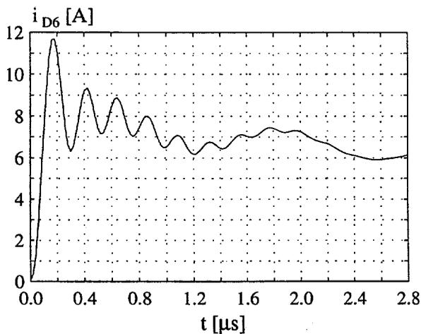
Fig. 5.39: The current in  $D_6$  during turn-on and the first part of the on-state at  $I_{Load} = 1$  mA.
