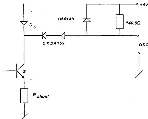
Fig. 5.15: The measuring circuit used when measuring the on-state power losses in the transistor.
