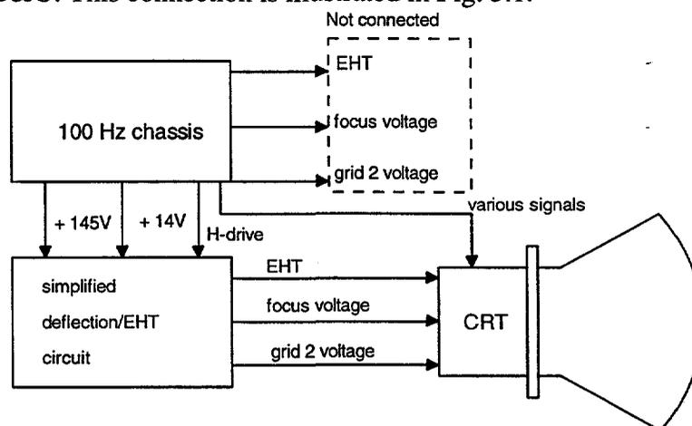
Fig. 3.1: Diagram showing the parallel connection of the 100 Hz chassis and the simplified deflection/EHT circuit.
