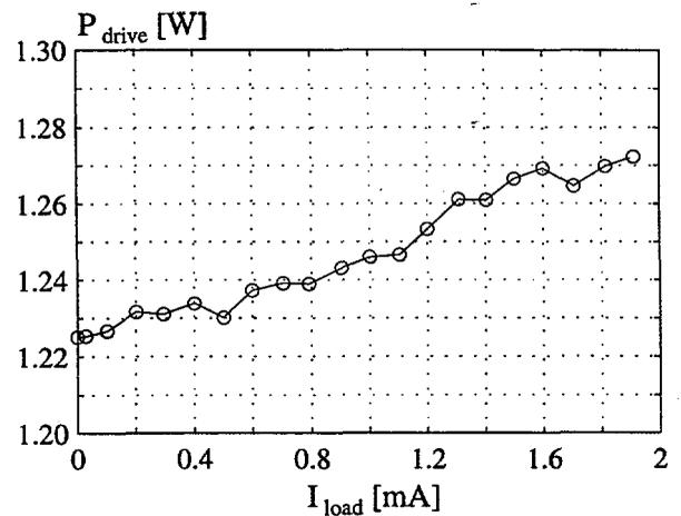
Fig. 5.25: The power to the drive circuit.
