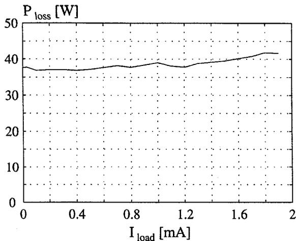
Fig. 5.7: The total power loss in the deflection/EHT circuit.
