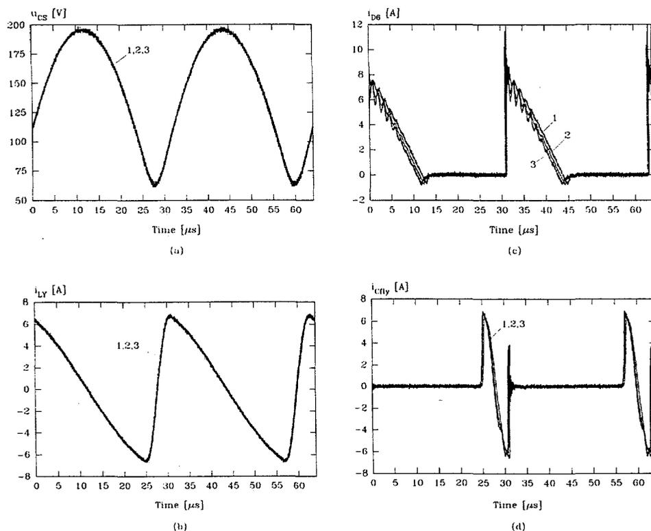
Fig. 3.7: The voltage and the current waveforms in the deflection circuit at 1:  $I_{\text{Load}} = 0 \text{ mA}$ , 2:  $I_{\text{Load}} = 1 \text{ mA}$ , and 3:  $I_{\text{Load}} = 2 \text{ mA}$ . (a) the voltage across the S-capacitor,  $C_S$ , (b) the deflection current, (c) the current through the diode,  $D_6$ , (d) the current through the flyback capacitor  $C_{\text{fly}}$ .
