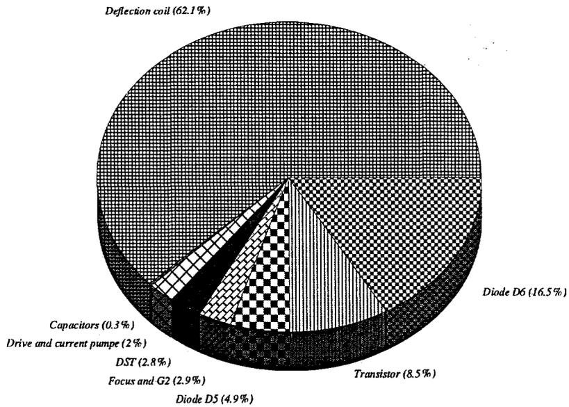
Fig. 5.51: The power losses in the deflection/EHT circuit at no load where the total power loss is 38.1 W. The losses are split up into the individual components in the circuit.
