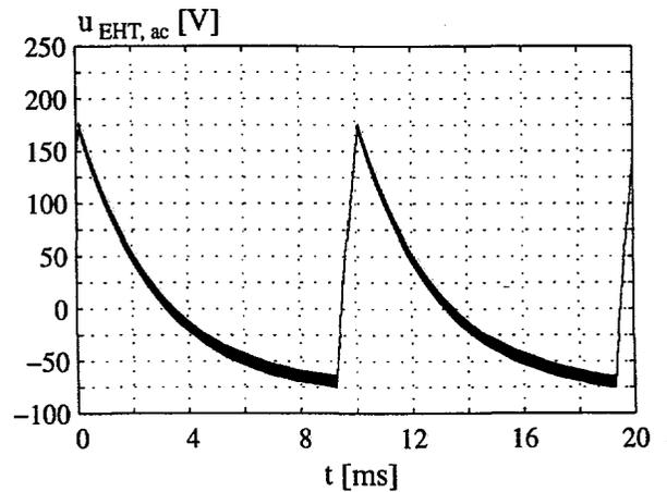
Fig. 4.27: The simulated a.c. content of the EHT at  $I_{Load} = 1 \text{ mA}$ .
