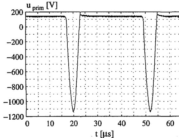
Fig. 5.45: The primary voltage of the DST at  $I_{Load} = 1 \text{ mA}$ . The measurement is performed on the circuit described in chapter 3.
