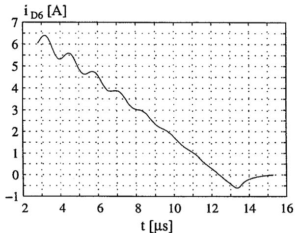
Fig. 5.40: The current in  $D_6$  during the last part of the on-state and the turn-off at  $I_{Load} = 1$  mA.
