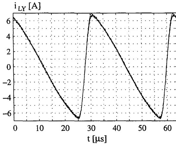
Fig. 4.18: The measured and the simulated deflection current at  $I_{Load} = 1 \text{ mA}$ .
