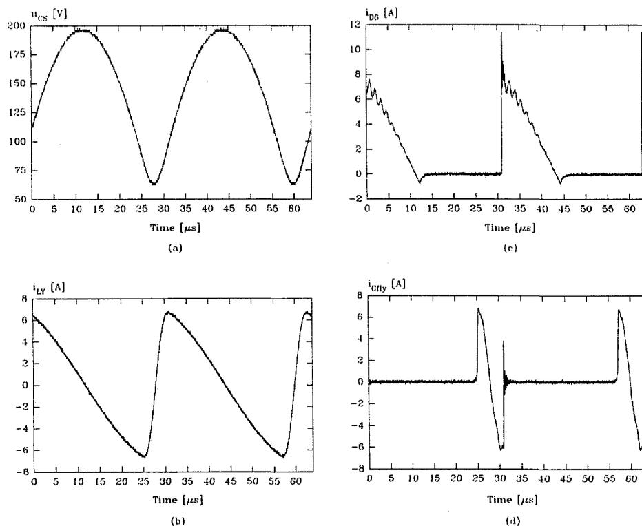
Fig. 3.6: The voltage and the current waveforms in the deflection circuit at  $I_{Load} = 1$  mA. (a) the voltage across the S-capacitor,  $C_S$ , (b) the deflection current, (c) the current through the diode,  $D_6$ , (d) the current through the flyback capacitor  $C_{fy}$ .
