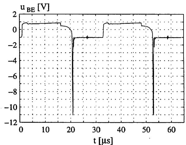
Fig. 5.14: The base-emitter voltage of the transistor at  $I_{Load} = 1$  mA.
