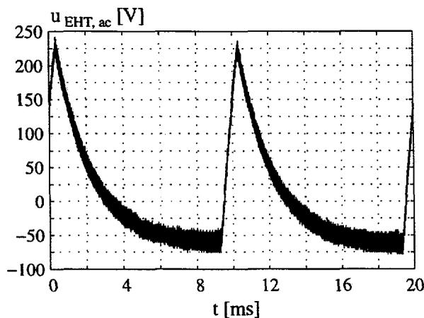
Fig. 4.13: The measured a.c. content of the EHT at  $I_{Load} = 1 \text{ mA}$ .
