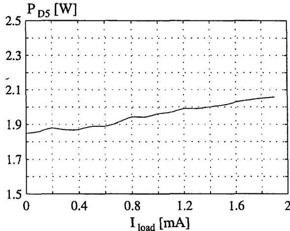
Fig. 5.43: The power losses in the diode  $D_5$ .
