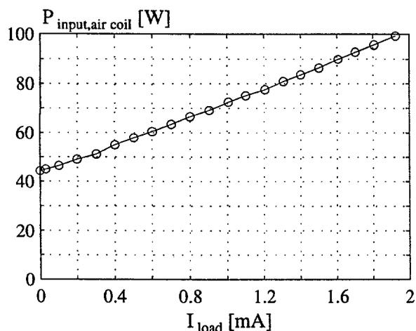
Fig. 5.34: The input power to the deflection/EHT circuit with the deflection coil replaced by the air coil.
