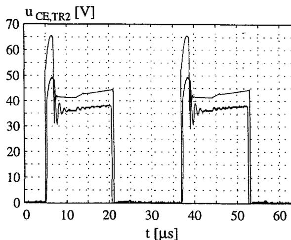
Fig. 4.31: The measured and the simulated collector-emitter voltage for transistor TR2 at  $I_{Load} = 1 \text{ mA}$ .
