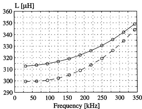
Fig. 5.31: The inductance of the deflection coils ( --: air coil, -: deflection coil).
