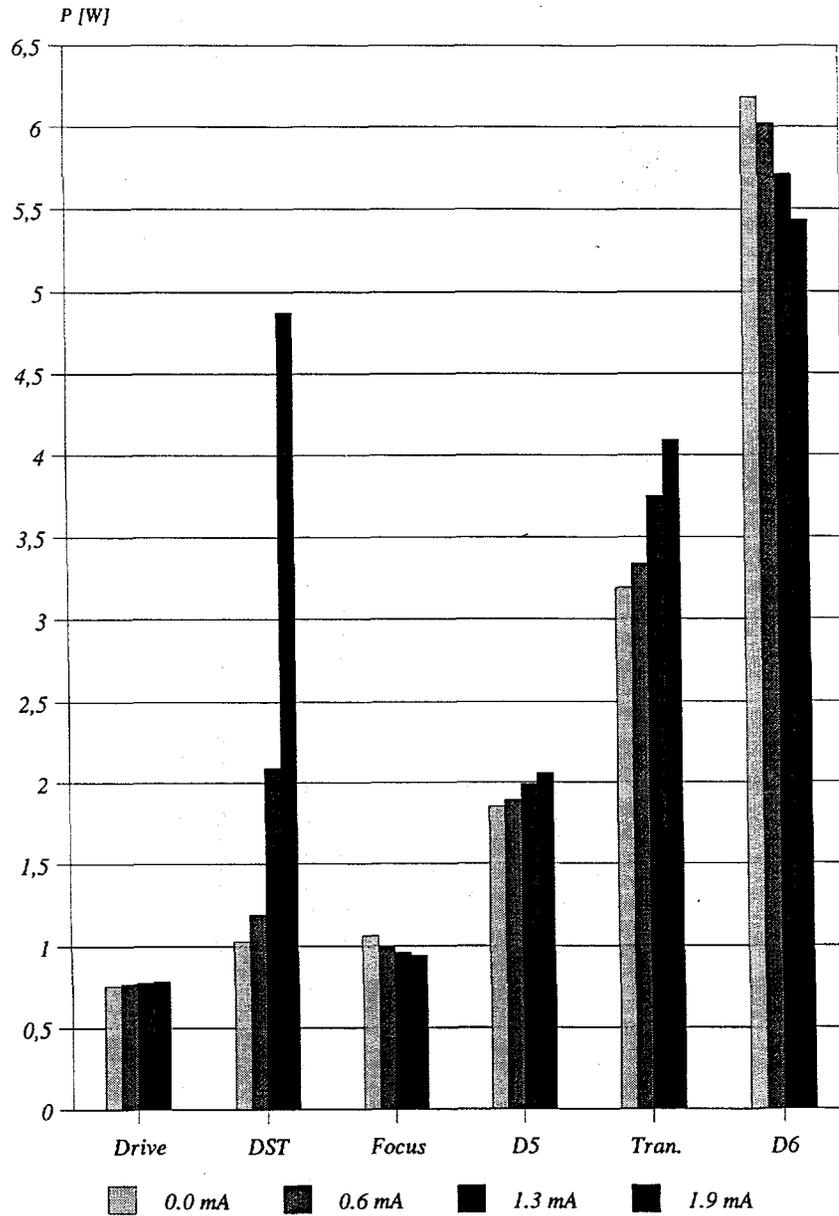
Fig. 5.55: The measured power loss in the individual components at the four different load currents. The power losses in the capacitors and the deflection coil are considered independent of the load current and are therefore not shown.
