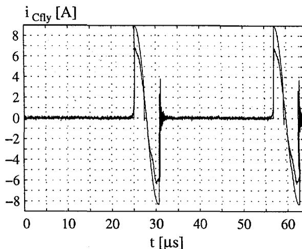
Fig. 4.4: The measured and the simulated current through the flyback capacitor at  $I_{Load} = 1 \text{ mA}$ .
