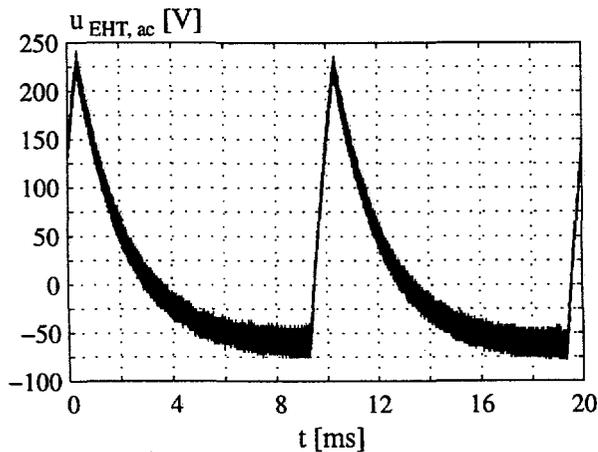
Fig. 4.26: The measured a.c. content of the EHT at  $I_{Load} = 1 \text{ mA}$ .
