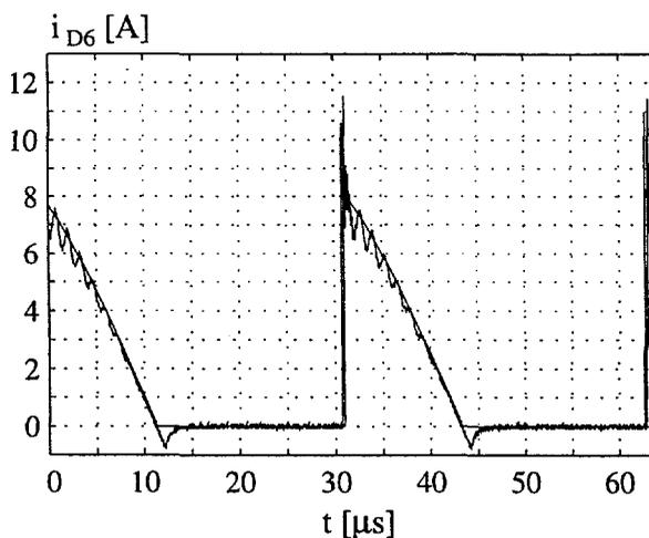
Fig. 4.6: The measured and the simulated current through the diode  $D_6$  at  $I_{Load} = 1 \text{ mA}$ .
