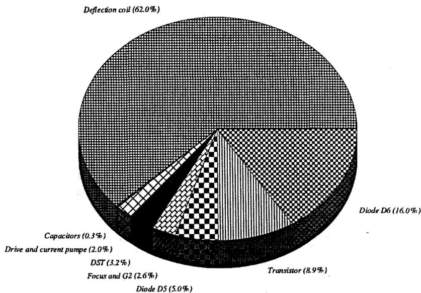
Fig. 5.52: The power losses in the deflection/EHT circuit at  $I_{Load} = 0.6$  mA where the total power loss is 38.2 W and the overall efficiency is 31.0 percent. The losses are split up into the individual components in the circuit.
