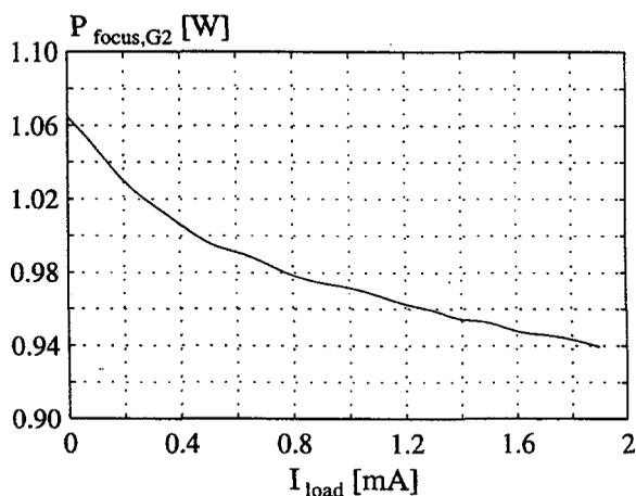
Fig. 5.49: The power losses in the focus and grid 2 potentiometers.
