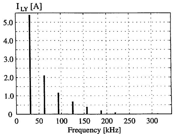
Fig. 5.33: The current harmonics in the deflection current  $I_{LY}$ .
