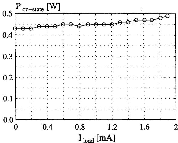
Fig. 5.28: The on-state losses in the transistor.
