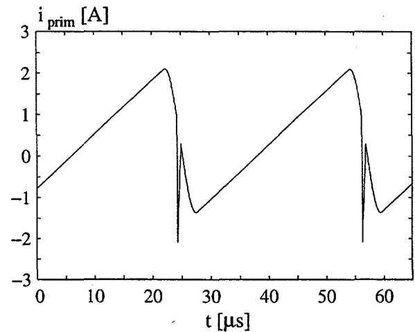
Fig. 2.9: The primary current of the DST,  $i_{prim}$  at  $I_{Load} = 1$  mA.
