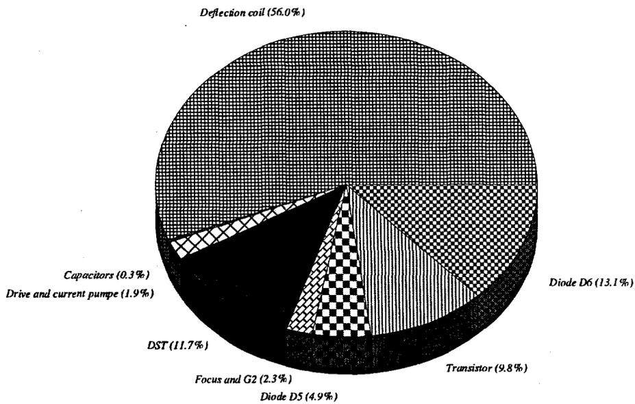
Fig. 5.54: The power losses in the deflection/EHT circuit at  $I_{Load} = 1.9 \text{ mA}$  where the total power loss is 42.2 W and the overall efficiency is 55.5 percent. The losses are split up into the individual components in the circuit.
