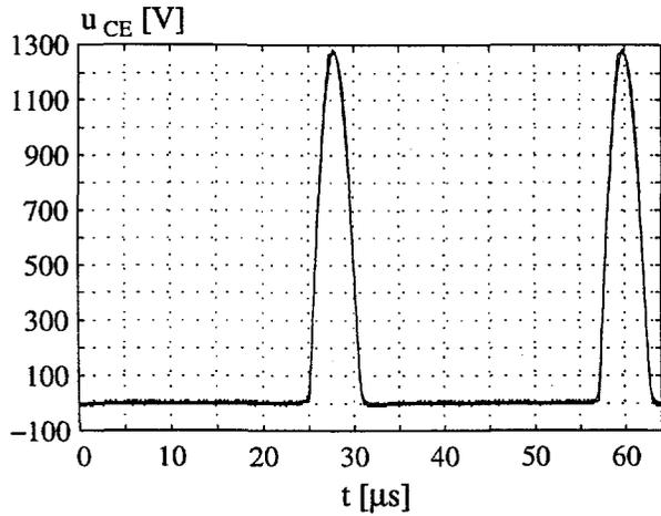
Fig. 4.22: The measured and the simulated collector-emitter voltage at  $I_{Load} = 1 \text{ mA}$ .
