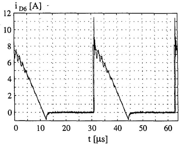
Fig. 4.19: The measured and the simulated current through the diode  $D_6$  at  $I_{Load} = 1 \text{ mA}$ .
