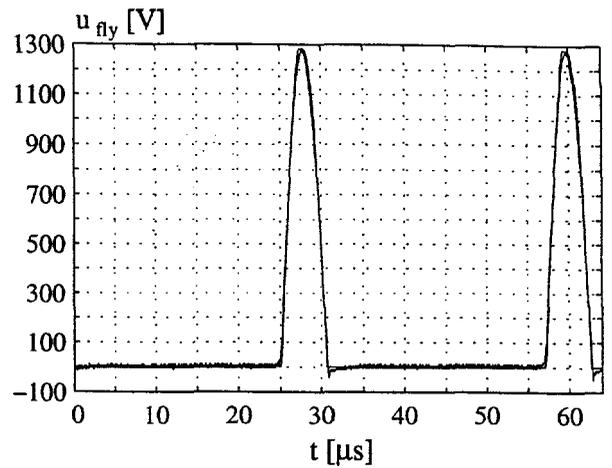
Fig. 4.10: The measured and the simulated flyback voltage at  $I_{Load} = 1 \text{ mA}$ .
