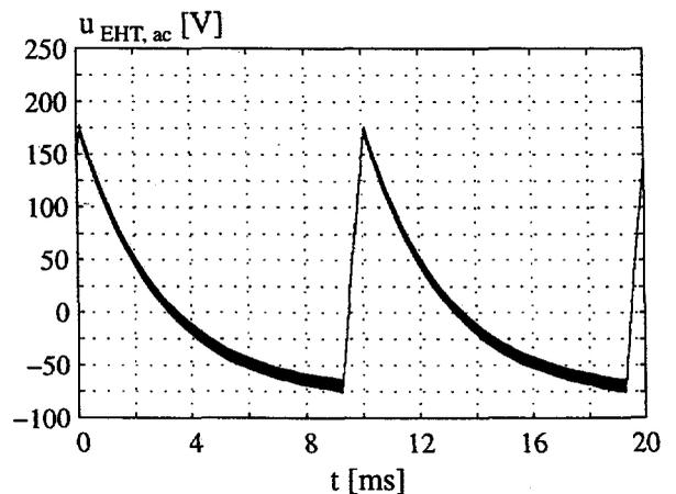
Fig. 4.14: The simulated a.c. content of the EHT at  $I_{Load} = 1 \text{ mA}$ .
