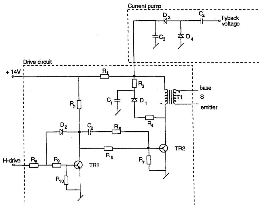
Fig. 2.4: The current pump and the drive circuit used in the simplified deflection/EHT circuit.
