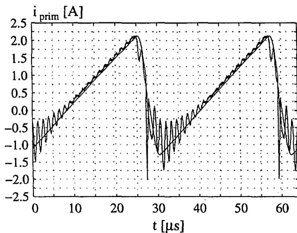
Fig. 4.20: The measured and the simulated primary current at  $I_{Load} = 1 \text{ mA}$ .
