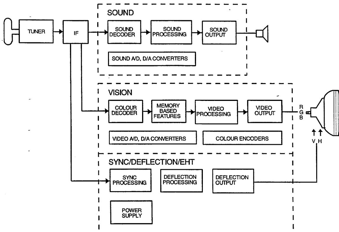
Fig. 2.1: Partitioning of a television set where only the basic functions are shown /8/.
