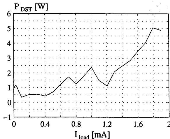
Fig. 5.50: The power losses in the diode split transformer including the power losses in the bleeder resistance.
