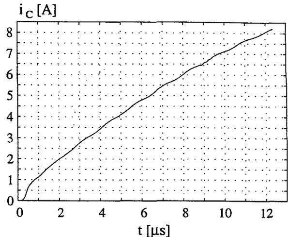
Fig. 5.18: The collector current during the on-state of the transistor at  $I_{Load} = 1 \text{ mA}$ .
