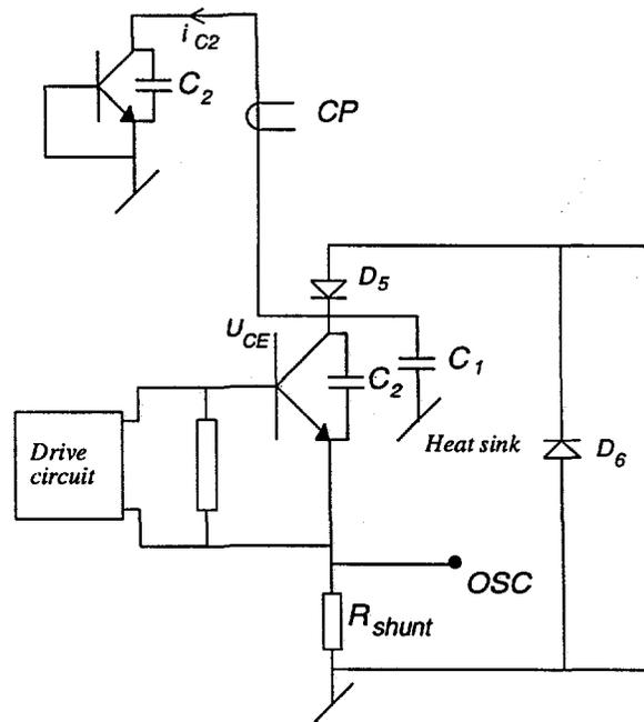
Fig. 5.19: Part of the deflection circuit illustrating the transistor's internal capacitor  $C_2$  and the capacitor  $C_1$  to the heat sink.
