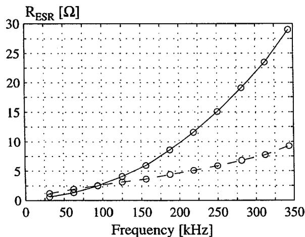
Fig. 5.32: The equivalent resistance of the deflection coils ( --: air coil, -: deflection coil).
