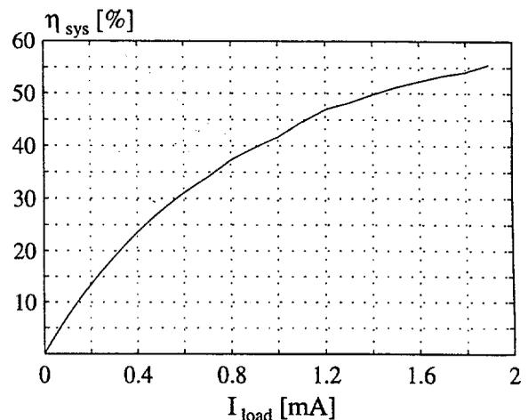
Fig. 5.8: The overall efficiency of the deflection/EHT circuit.
