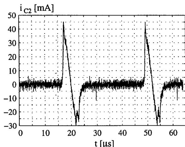
Fig. 5.20: The current through the internal capacitor  $C_2$  in the transistor at  $I_{Load} = 1 \text{ mA}$ .
