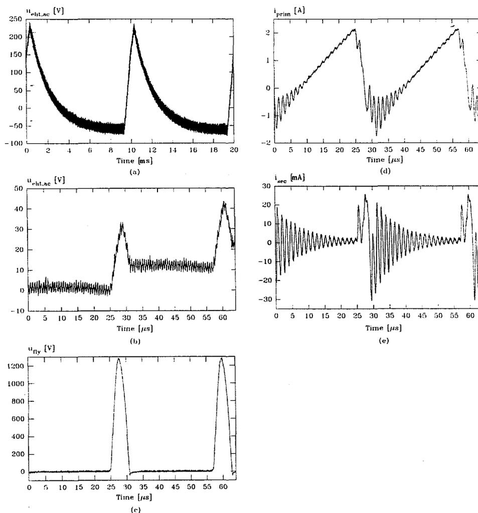
Fig. 3.8: The voltage and the current waveforms in the diode split transformer, DST, at  $I_{Load} = 1$  mA. (a) the a.c. content of the EHT, (b) the a.c. content of the EHT, (c) the flyback voltage, (d) the primary current, (e) the secondary current.
