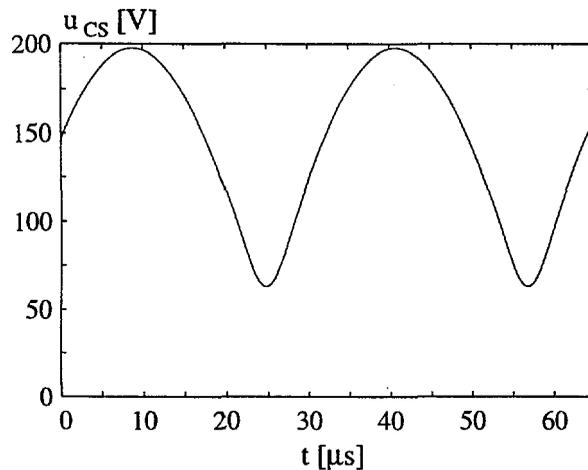
Fig. 2.8: The voltage across the S-capacitor,  $u_{CS}$  at  $I_{Load} = 1$  mA.
