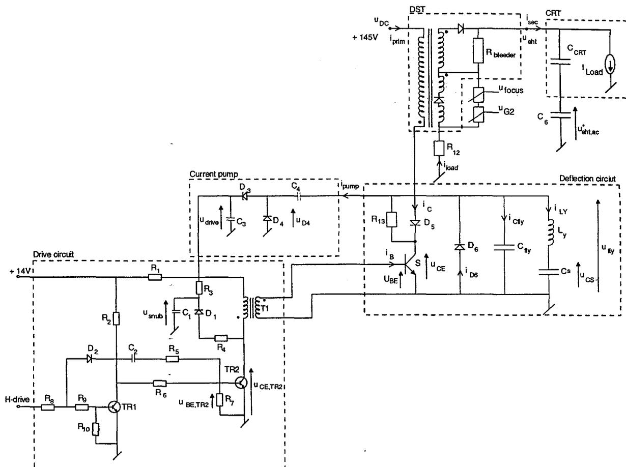
Fig. 3.2: Diagram of the built laboratory model of the simplified deflection/EHT circuit. A diagram with the values of the components is given in supplement 4.
