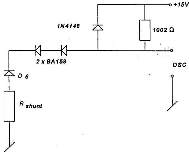
Fig. 5.38: The measuring circuit used when measuring the on-state and the turn-off power losses in the power diode  $D_6$ .
