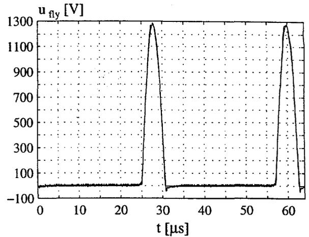
Fig. 4.23: The measured and the simulated flyback voltage at  $I_{Load} = 1 \text{ mA}$ .
