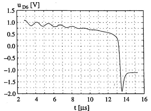
Fig. 5.42: The voltage of  $D_6$  during the last part of the on-state and the turn-off at  $I_{Load} = 1$  mA.
