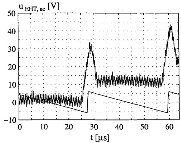
Fig. 4.25: The measured and the simulated a.c. content of the EHT at  $I_{Load} = 1 \text{ mA}$ .
