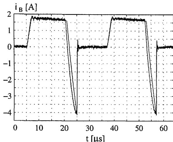
Fig. 4.28: The measured and the simulated base current to the transistor at  $I_{Load} = 1 \text{ mA}$ .
