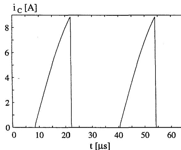
Fig. 2.10: The collector current in the transistor,  $i_C$  at  $I_{Load} = 1$  mA.
