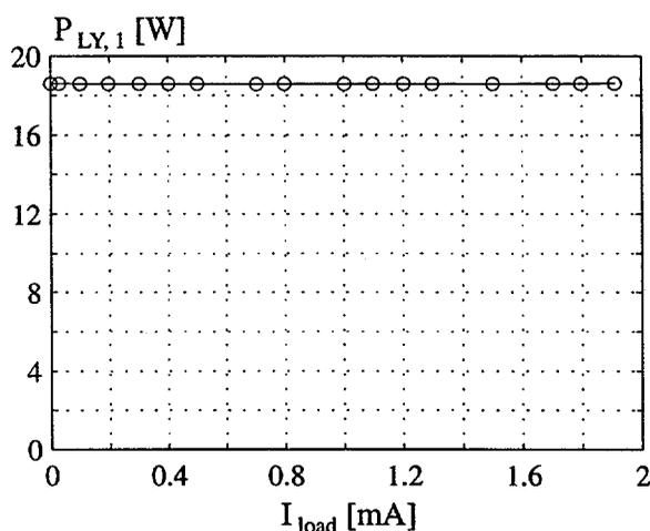
Fig. 5.36: The power losses in the deflection coil calculated from (5-15).
