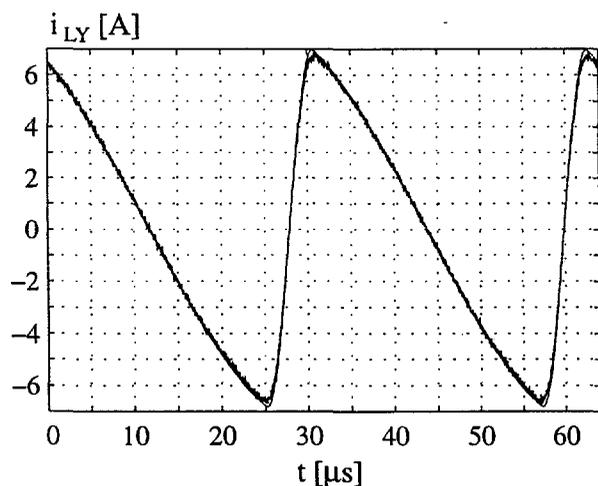
Fig. 4.5: The measured and the simulated deflection current at  $I_{Load} = 1 \text{ mA}$ .
