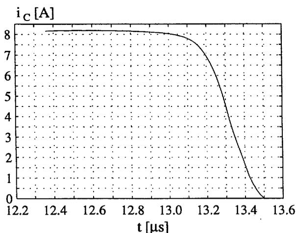
Fig. 5.22: The collector current during turn-off of the transistor at  $I_{Load} = 1 \text{ mA}$ .
