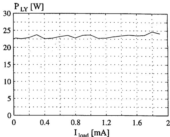
Fig. 5.35: The power losses in the deflection coil calculated by use of the air coil.
