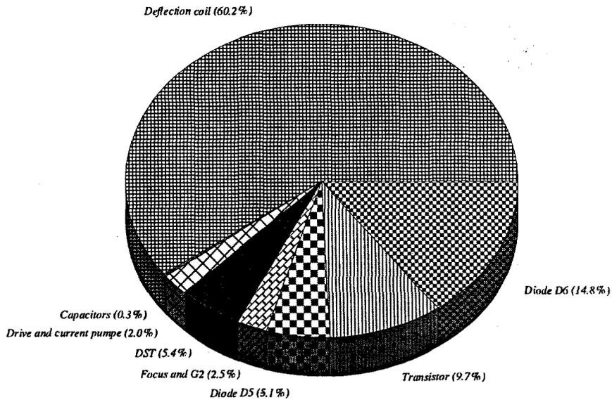
Fig. 5.53: The power losses in the deflection/EHT circuit at  $I_{Load} = 1.3 \text{ mA}$  where the total power loss is 38.7 W and the overall efficiency is 48.1 percent. The losses are split up into the individual components in the circuit.
