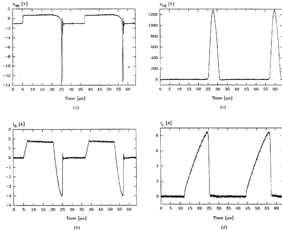
Fig. 3.4: The voltage and the current waveforms of the deflection transistor at  $I_{Load} = 1 \text{ mA}$ . (a) the base-emitter voltage, (b) The base current, (c) the collector-emitter voltage, (d) the collector current.
