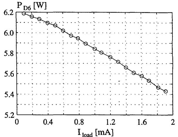
Fig. 5.44: The power losses in the diode  $D_6$ .
