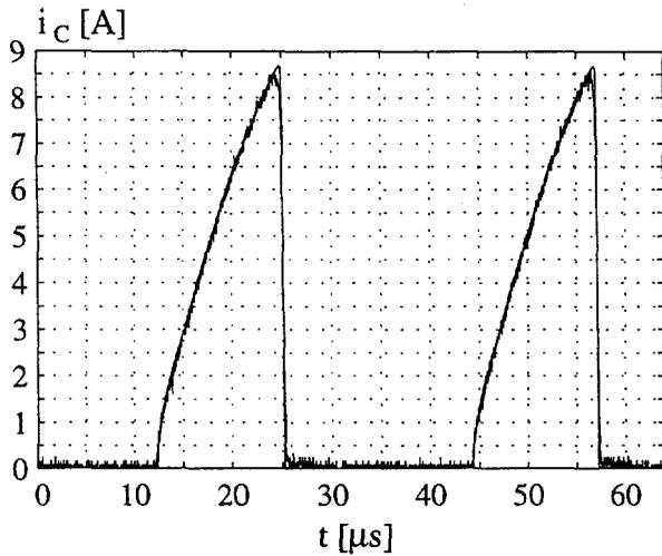
Fig. 4.16: The measured and the simulated collector current at  $I_{Load} = 1 \text{ mA}$ .
