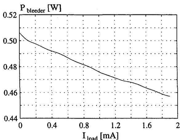
Fig. 5.48: The power losses in the bleeder resistance.
