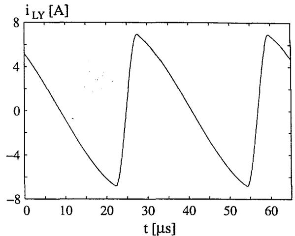
Fig. 2.7: The deflection current  $i_{LY}$  at  $I_{Load} = 1$  mA.
