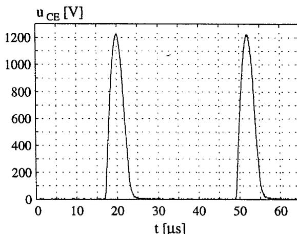
Fig. 5.21: The collector-emitter voltage at  $I_{Load} = 1 \text{ mA}$ .
