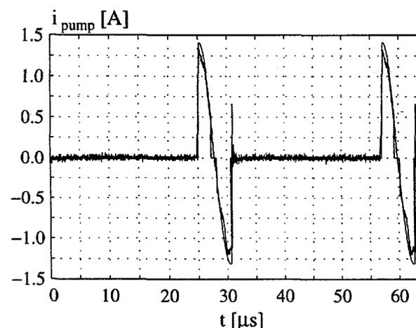
Fig. 4.32: The measured and the simulated current to the current pump at  $I_{Load} = 1 \text{ mA}$ .
