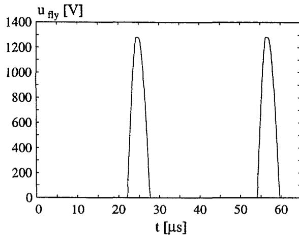
Fig. 2.6: The flyback voltage  $u_{fly}$  at  $I_{Load} = 1$  mA.
