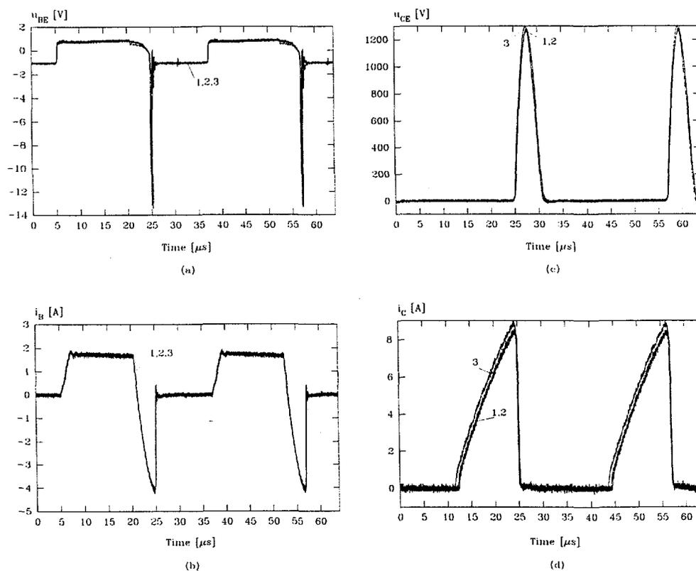
Fig. 3.5: The voltage and the current waveforms of the deflection transistor at 1:  $I_{\text{Load}} = 0 \text{ mA}$ , 2:  $I_{\text{Load}} = 1 \text{ mA}$ , and 3:  $I_{\text{Load}} = 2 \text{ mA}$ . (a) the base-emitter voltages, (b) the base currents, (c) the collector-emitter voltages, (d) the collector currents.
