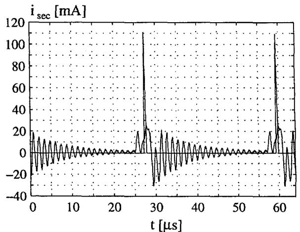
Fig. 4.21: The measured and the simulated secondary current at  $I_{Load} = 1 \text{ mA}$ .
