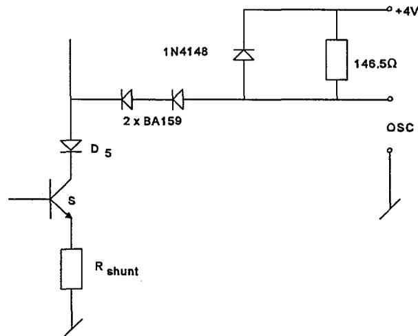
Fig. 5.37: The measuring circuit used when measuring the on-state power losses in the power diode  $D_5$ .
