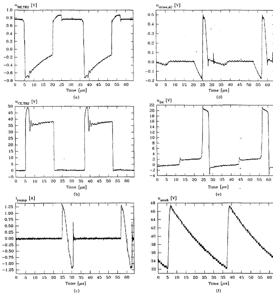
Fig. 3.3: The voltage and the current waveforms in the drive circuit at  $I_{Load} = 1 \text{ mA}$ . (a) the base-emitter voltage for the transistor, TR2, (b) the collector-emitter voltage for the transistor, TR2, (c) the current to the current pump, (d) the a.c. content of the voltage to the drive circuit where the d.c. content is approximately 19.7 V, (e) the voltage across the diode,  $D_4$ , (f) the voltage across the snubber capacitor,  $C_1$ .
