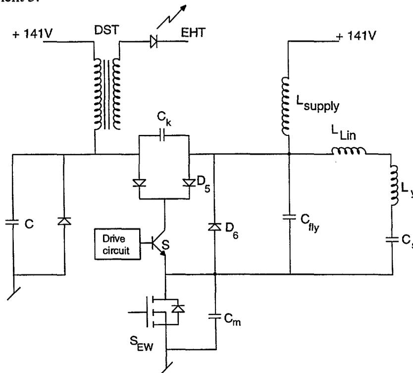
Fig. 2.2: Principal diagram of the horizontal deflection circuit and the EHT generator in use at B&O.
