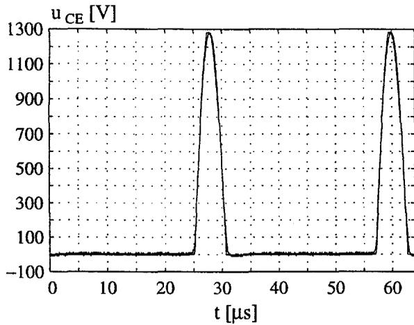
Fig. 4.9: The measured and the simulated collector-emitter voltage at  $I_{Load} = 1 \text{ mA}$ .
