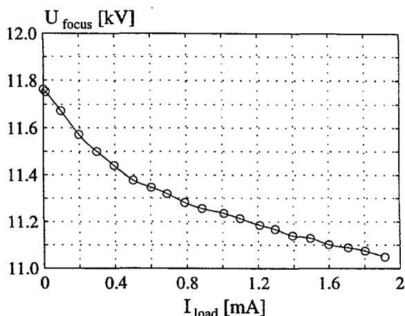
Fig. 5.47: The voltage to the focus and the grid 2 potentiometers.
