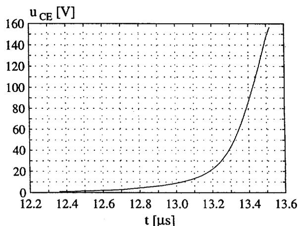
Fig. 5.23: The collector-emitter voltage during turn-off of the transistor at  $I_{Load} = 1 \text{ mA}$ .
