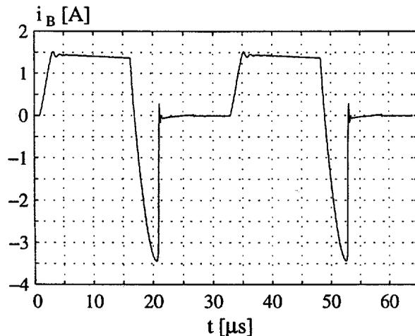
Fig. 5.13: The current to the base of the transistor at  $I_{Load} = 1$  mA.
