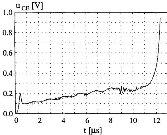
Fig. 5.17: The collector-emitter voltage during the on-state of the transistor at  $I_{Load} = 1 \text{ mA}$ .
