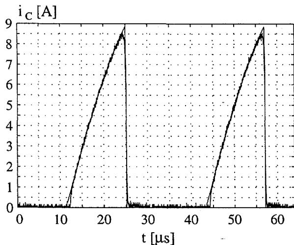
Fig. 4.3: The measured and the simulated collector current at  $I_{Load} = 1 \text{ mA}$ .
