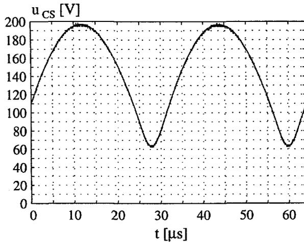
Fig. 4.24: The measured and the simulated voltage across the S-capacitor at  $I_{Load} = 1 \text{ mA}$ .
