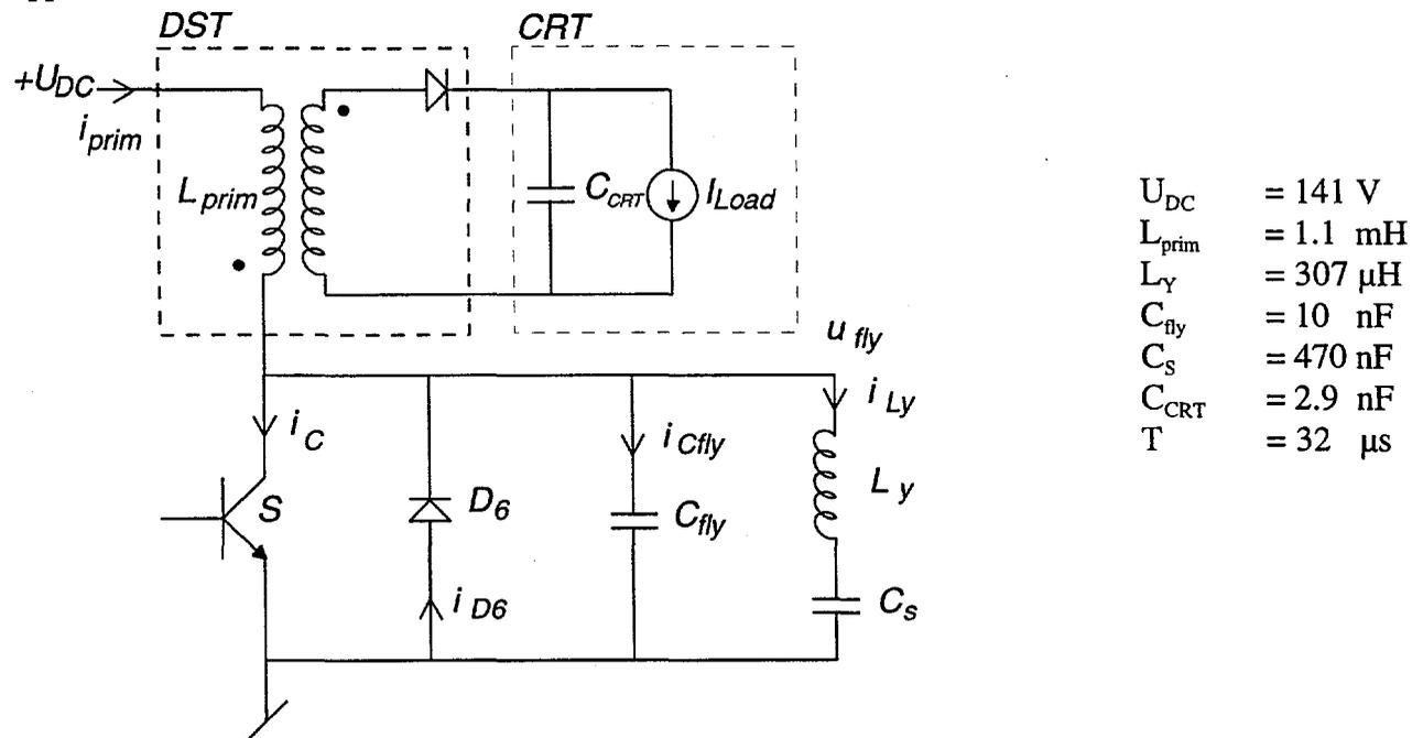
Fig. 2.5: A simplified diagram of the deflection/EHT circuit.
