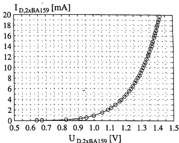
Fig. 5.16: The "diode characteristic" for the series connection of the two diodes BA159.
