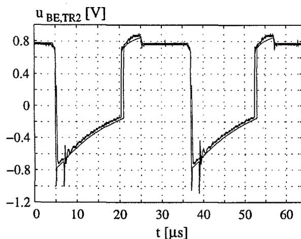
Fig. 4.30: The measured and the simulated base-emitter voltage for transistor TR2 at  $I_{Load} = 1 \text{ mA}$ .
