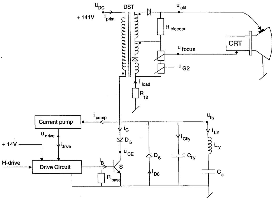
Fig. 5.1: The simplified deflection/EHT circuit in which the power losses are measured.
