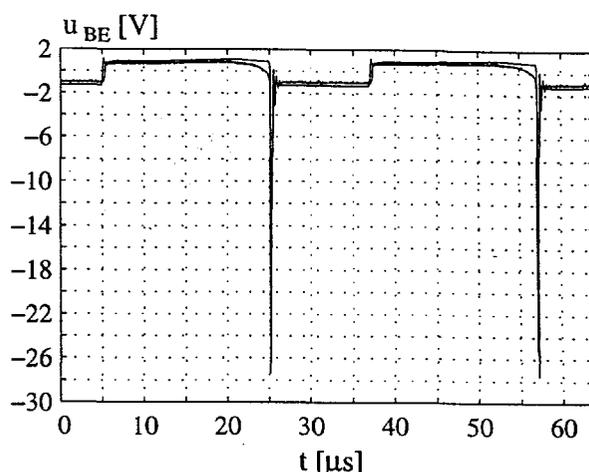
Fig. 4.29: The measured and the simulated base-emitter voltage at  $I_{Load} = 1 \text{ mA}$ .
