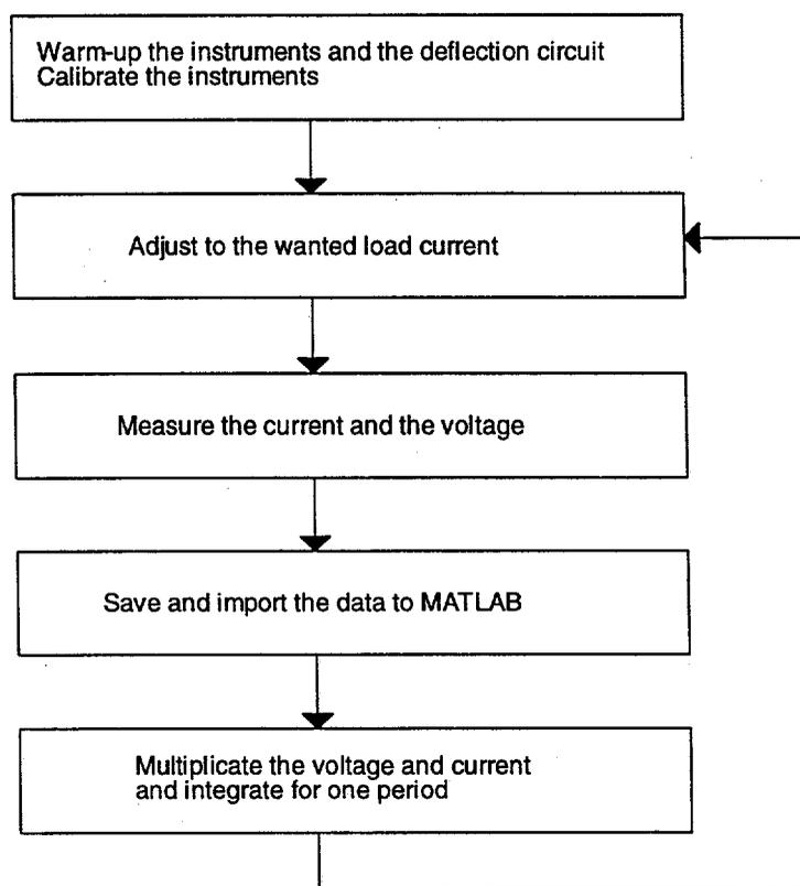
Fig. 5.2: The general measuring process when using the digital storage oscilloscope.
