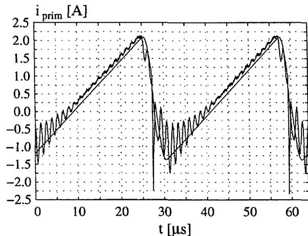
Fig. 4.7: The measured and the simulated primary current at  $I_{Load} = 1 \text{ mA}$ .
