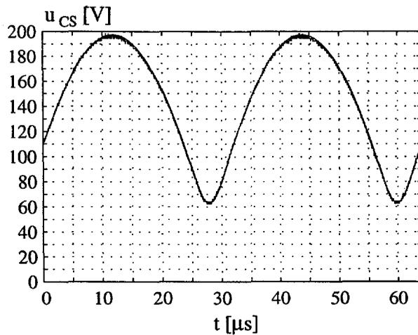
Fig. 4.11: The measured and the simulated voltage across the S-capacitor at  $I_{Load} = 1 \text{ mA}$ .
