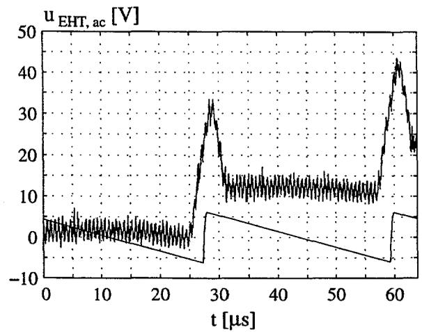
Fig. 4.12: The measured and the simulated a.c. content of the EHT at  $I_{Load} = 1 \text{ mA}$ .
