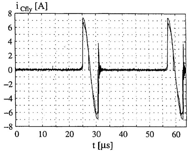
Fig. 4.17: The measured and the simulated current in the flyback capacitor at  $I_{Load} = 1 \text{ mA}$ .
