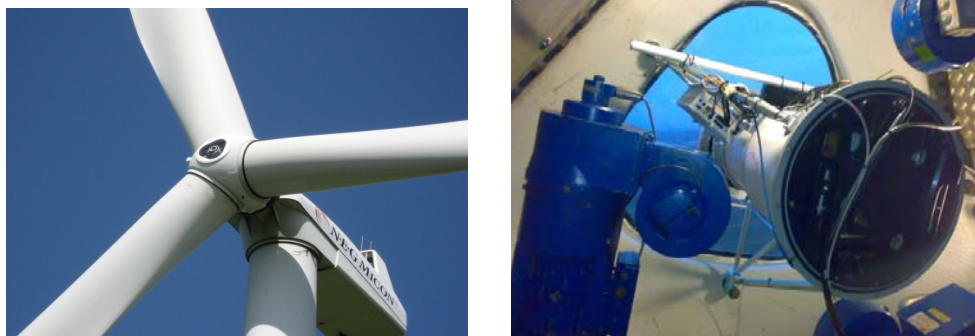
Figure 1 Photograph of the NM 80 wind turbine. Here it is visible the optical head of the QinetiQ's (Natural Power) ZephIR lidar in the tip of the wind turbine spinner (left). In addition it can be seen the interior of the spinner where the lidar was mounted (right).
