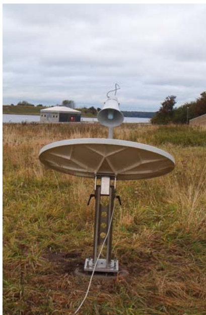
Figure 1. The Heimdall sodar transmitter at Risø. The speaker is located in the focus of the antenna disk.
