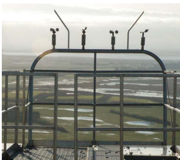
Figure 1 Arrangement of nacelle anemometry on the back of the nacelle of modern wind turbines. The instruments are typically mounted on a reasonably solid support structure with lightning protection covering the instruments and with redundant mounting of instruments
