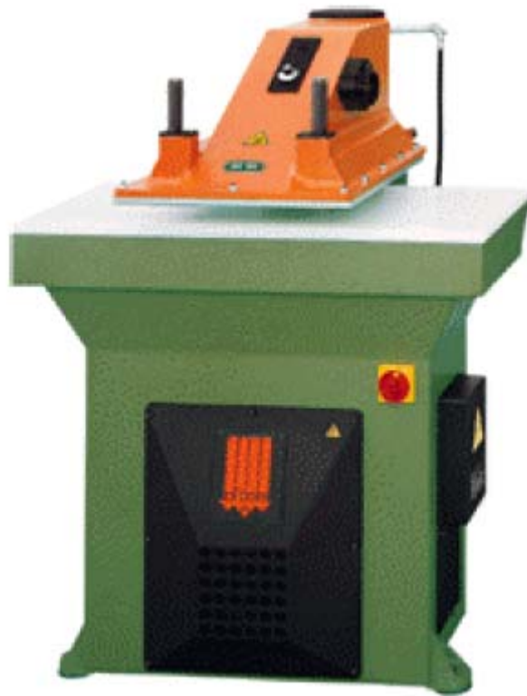
Figure 12. ATOM clicker press for stamping out membranes, electrodes and seals.
