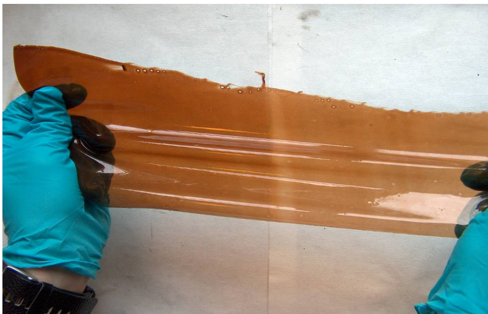
Figure 5. Sample of direct cast PBI membranes containing 93 wt% phosphoric acid.
