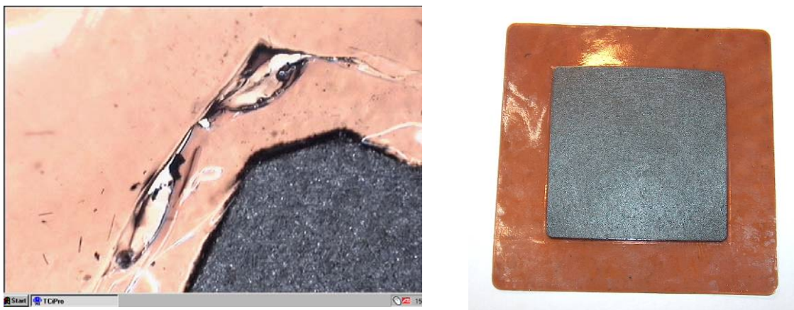
Figure 11. Left: a MEA (from before the project) without edge sealing showing the characteristic holes along the electrode edge. Right: a MEA with applied edge sealing and hot pressed using the new tool.
