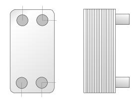
Figure 11. 6 Brazed plate heat exchanger.
