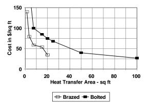
Figure 11.8 Plate heat exchanger cost comparison.
