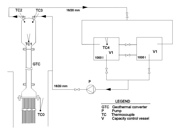
Figure 11.10 Schematic of experimental loop (Cannaviello, et al., 1982).
