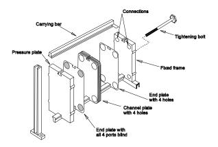
Figure 11.1 The plate heat exchanger.
