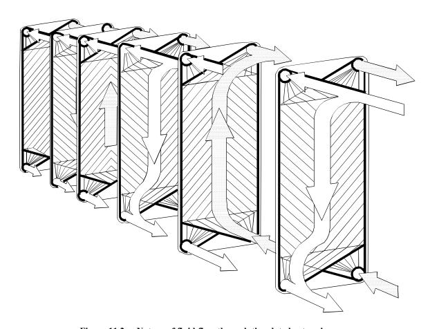
Figure 11.2 Nature of fluid flow through the plate heat exchanger.
