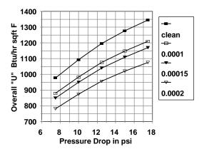
Figure 11.4 Performance of plate heat exchangers.
