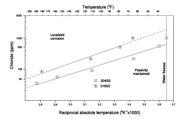
Figure 11.3 Chloride required to produce localized corrosion of Type 304 and Type 316 as a function of temperature (Efird and Moller, 1978).
