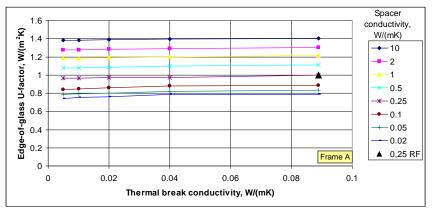
Figure 8. Edge-of-glass U-factor as a function of thermal break conductivity (horizontal axis) and spacer conductivity (various line types) for Frame A (thermally broken aluminum).
