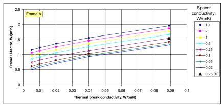
Figure 7. Frame U-factor as a function of thermal break conductivity (horizontal axis) and spacer conductivity (various line types) for Frame A (thermally broken aluminum).
