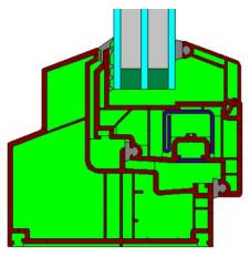
Figure 6. Cross-section of Frame E. The brown areas show the PVC skeleton of the frame, and the light green areas show air cavities. The blue areas show the supporting steel and the continuous parts of the hardware used for opening the frame.
