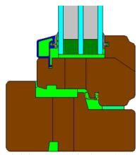
Figure 5. Cross-section of Frame D. Solid core wood is shown in brown. Air cavities are shown in light green.
