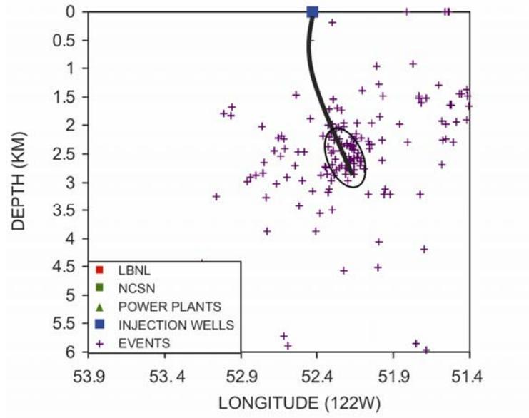
Figure 4. E-W projection through a 6 km cube containing MEQ hypocenters of magnitude 0.8 or larger during 1 year of injection at Aidlin 11 (from Majer and Peterson (2007)).
