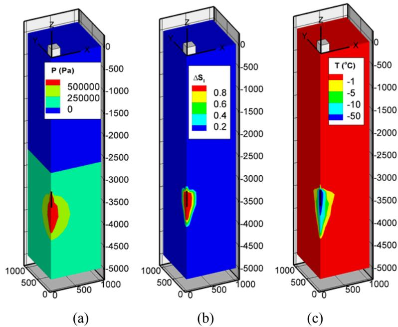
Figure 5. Simulation results of after 1 year of water injection at Aidlin 11: Changes in (a) fluid pressure, (b) liquid saturation, (c) temperature after 1 year of injection.
