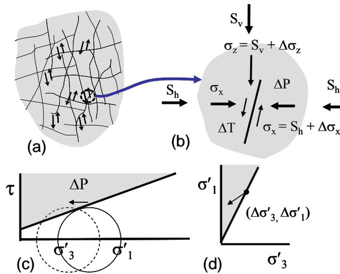
Figure 3. Illustration of the approach for failure analysis to evaluate the potential for induced seismicity at The Geysers (a) Highly fractured rock with randomly oriented fractures, (b) Changes in stress on one fracture plane, (c) Movements of Mohr's circle as a result of increased fluid pressure within a fracture plane for a critically stressed fracture, and (d) corresponding stress path in the  $(\sigma'_1, \sigma'_3)$  plane.
