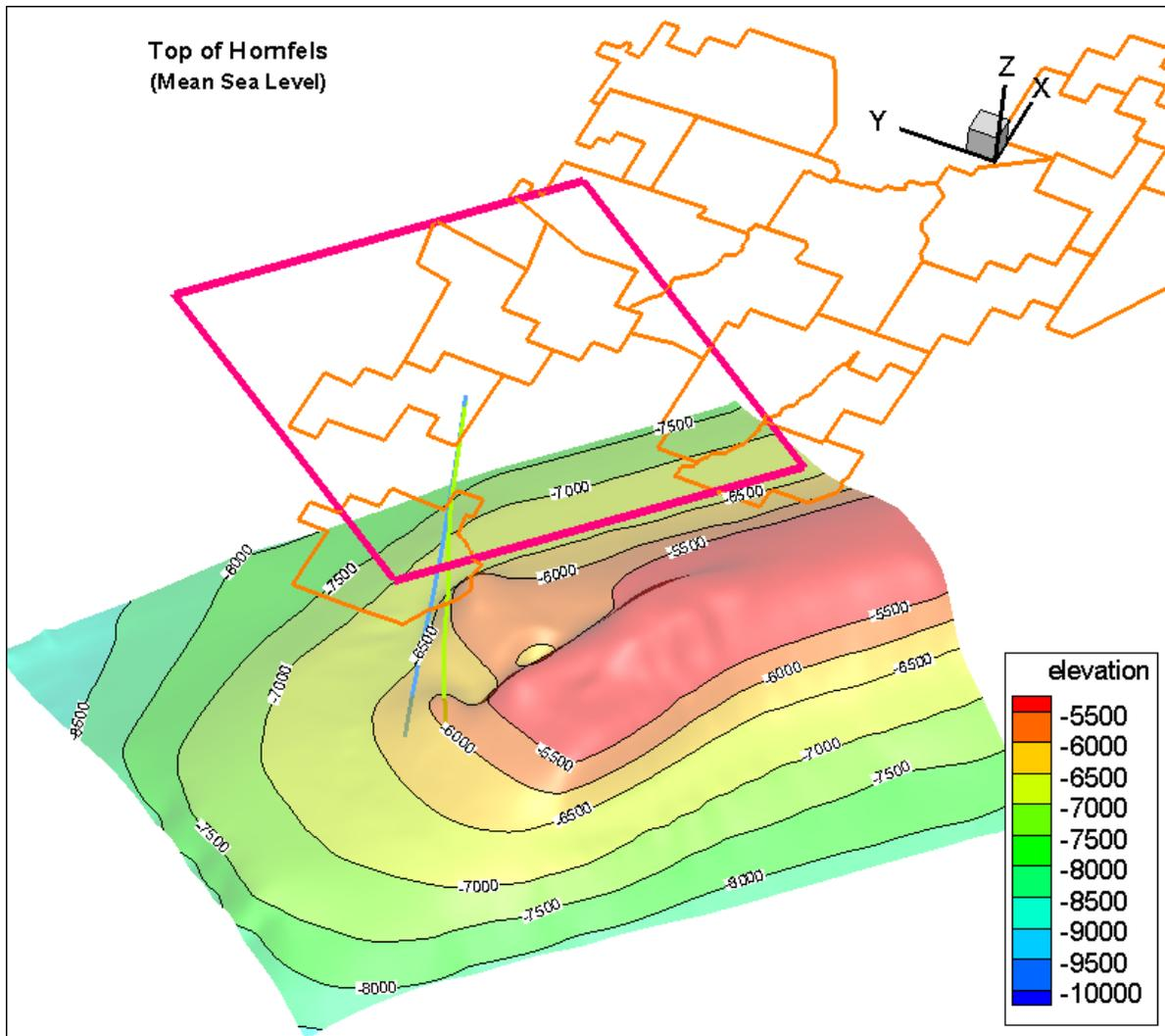
Figure 2. Three dimensional view of the top of hornfels showing PS-31 and P-32 wells.
